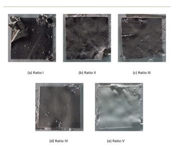
Fig. 1 Single layer sintered WSPC and Co-PES samples prepared using different mass ratios of walnut shell powder and Co-PES.
