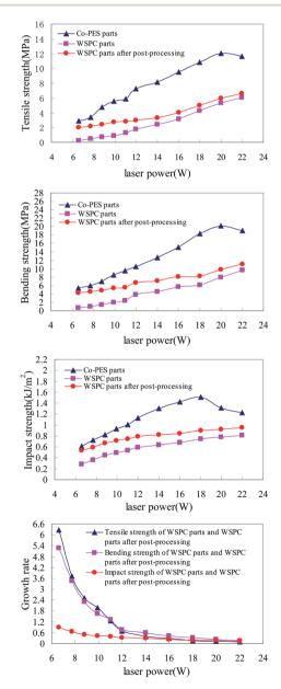
**Fig. 8** Change curves of mechanical properties and growth rate of Co-PES parts, WSPC parts and WSPC parts after post-processing with the change in laser power.
