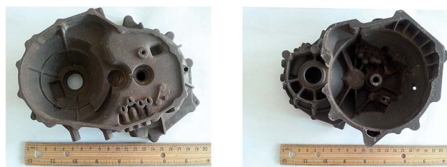
(a) Outside of the chassis (b) Inside of the chassis Fig. 5 WSPC demonstration part after post-processing.
