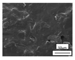
**Fig. 7** SEM photo of the cross-section of the WSPC laser sintered part after post-processing magnified by 500.
