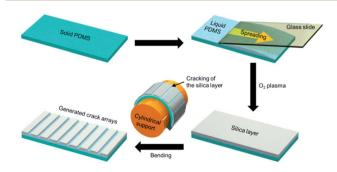
Fig. 1 A schematic diagram of the fabrication steps for periodic crack patterns on the liquid-PDMS-covered elastomeric substrate formed by oxygen plasma and bending.
