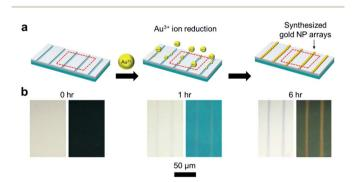
Fig. 2 In situ synthesis of gold NPs along the cracked lines on the PDMS substrate. (a) A schematic illustration of the synthesis of gold NPs by crack templated reduction lithography (CTRL). (b) The transmittance (left) and reflection (right) optical images of the perpendicular crack lines at the same region during the 6 h reduction reaction.
