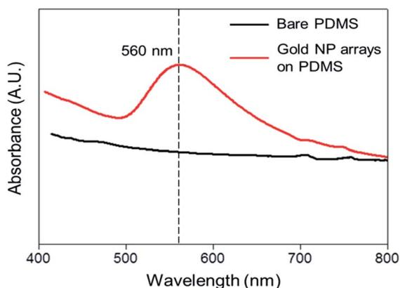
Fig. 4 UV-visible spectra of a bare PDMS substrate and the gold NP arrays on PDMS.
