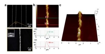
Fig. 3 Morphological characteristics of the synthesized gold NP arrays. (a) FE-SEM image of the aligned gold nanoparticle composite wire arrays. Inset image shows the cross-sectional view and the scale bar is 1  $\mu$ m. (b) AFM image of the gold NP array with a scan size of 5  $\times$  5  $\mu$ m. The inserted z-scale bar corresponds to 0 to 200 nm from bottom to top. (c) AFM 3D view of the produced gold NP array with a scan size of  $5 \times 5 \mu m$ .
