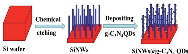
Fig. 1 The schematic diagram of the preparation process of SiNWs@*g*-C<sub>3</sub>N<sub>4</sub> QDs. SiNW was represented by blue column, and the *g*-C<sub>3</sub>N<sub>4</sub> QDs were represented by yellow balls.
