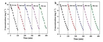
Fig. 7 Consecutive runs in the photoelectrocatalytic degradation of 4-chlorophenol ( $C_0=10~{\rm mg~L^{-1}}$ ) for (a) SiNWs photocathode and (b) SiNWs@g-C $_3$ N $_4$  QDs photocathode ( $-1.2~{\rm V}$  vs. SCE) under visible light irradiation ( $\lambda$  > 400 nm,  $I=100~{\rm mW~cm^{-2}}$ ).
