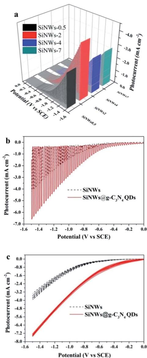
Fig. 5 Photoelectrochemical properties: (a)  $I$ - $V$  curves of SiNWs photocathodes with various etching times; (b)  $I$ - $V$  curves of SiNWs and SiNWs@g-C<sub>3</sub>N<sub>4</sub> QDs photocathodes and (c) 10 cycles of cyclic voltammetry curves of SiNWs and SiNWs@g-C<sub>3</sub>N<sub>4</sub> QDs photocathodes in 0.5 M H<sub>2</sub>SO<sub>4</sub> solution under xenon lamp illumination (100 mW cm<sup>-2</sup>).
