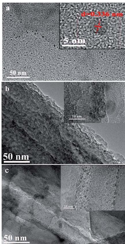
Fig. 3 TEM images of (a)  $g\text{-C}_3\text{N}_4$  QDs (inset: HRTEM image, scale bar: 5 nm), (b) pristine SiNWs (inset: HRTEM image, scale bar: 10 nm), (c) SiNWs@ $g\text{-C}_3\text{N}_4$  QDs (inset: HRTEM image, scale bar: 10 nm).
