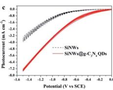
Fig. 5 Photoelectrochemical properties: (a) I-V curves of SiNWs photocathodes with various etching times; (b) I-V curves of SiNWs and SiNWs@g-C<sub>3</sub>N<sub>4</sub> QDs photocathodes and (c) 10 cycles of cyclic voltammetry curves of SiNWs and SiNWs@g-C<sub>3</sub>N<sub>4</sub> QDs photocathodes in 0.5 M H<sub>2</sub>SO<sub>4</sub> solution under xenon lamp illumination (100 mW cm<sup>-2</sup>).
