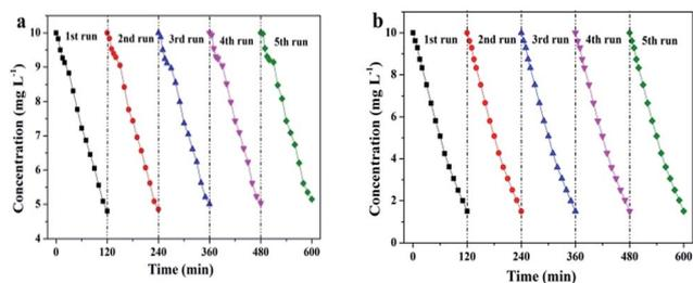
Fig. 7 Consecutive runs in the photoelectrocatalytic degradation of 4-chlorophenol ( $C_0 = 10 \text{ mg L}^{-1}$ ) for (a) SiNWs photocathode and (b) SiNWs@g-C<sub>3</sub>N<sub>4</sub> QDs photocathode ( $-1.2 \text{ V vs. SCE}$ ) under visible light irradiation ( $\lambda > 400 \text{ nm}$ ,  $I = 100 \text{ mW cm}^{-2}$ ).
