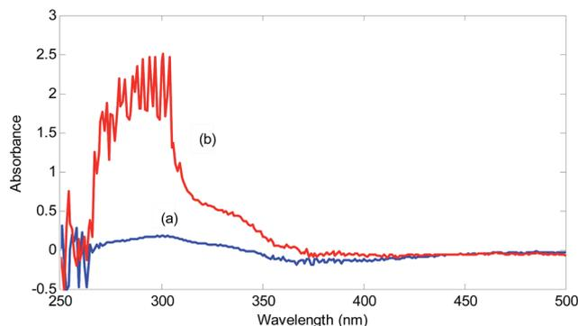
Fig. 2 Spectra of the reagent blank ( $5.00 \times 10^{-4} \text{ mol L}^{-1}$  NQS and  $1.00 \times 10^{-2} \text{ mol L}^{-1}$  hydrochloric acid) in the presence of  $2.00 \text{ mg L}^{-1}$  hydrogen sulfide in (a) deionized water and (b) urine sample.
