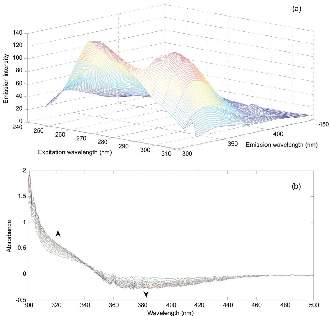
Fig. 6 (a) EEM spectra recorded for Milk 1 sample after addition of standard in the presence of the reagents (0.18 mL concentrated sulfuric acid,  $\text{Fe}^{2+}$   $6.0 \times 10^{-4}$  mol L<sup>-1</sup> and phenol 150.0 mg L<sup>-1</sup>) and (b) kinetic UV-Vis spectra recorded for urine sample during reaction of hydrogen sulfide in the presence of reagents ( $5.00 \times 10^{-4}$  mol L<sup>-1</sup> NQS and  $1.00 \times 10^{-2}$  mol L<sup>-1</sup> hydrochloric acid).
