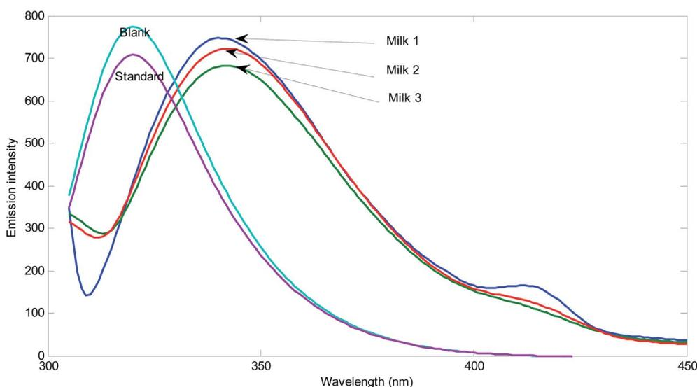
Fig. 1 Spectra of the reagent blank (0.18 mL concentrated sulfuric acid,  $\text{Fe}^{2+}$   $6.0 \times 10^{-4} \text{ mol L}^{-1}$  and phenol  $150.0 \text{ mg L}^{-1}$ ), reagent blank in the presence of  $5.0 \times 10^{-6} \text{ mol L}^{-1}$  of standard hydrogen peroxide, and different milk samples after addition of  $5.0 \times 10^{-6}$  (Milk 1),  $5.0 \times 10^{-6}$  (Milk 2), and  $1.0 \times 10^{-5}$  (Milk 3).
