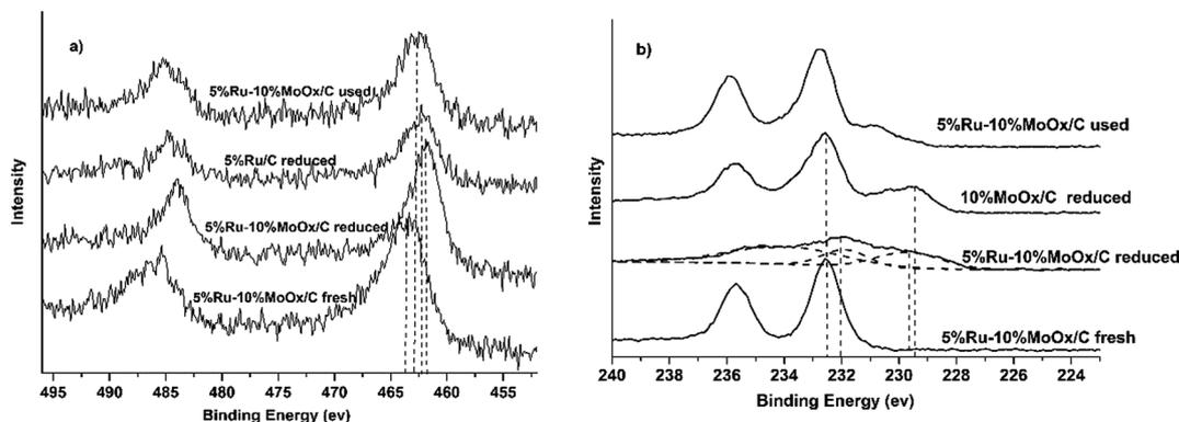
Fig. 2 XPS spectra of Ru– $MoO_x$ /C catalysts: (a) Ru 3p and (b) Mo 3d. 5% Ru–10%  $MoO_x$ /C fresh: the catalyst had not been reduced by  $H_2$ ; 5% Ru–10%  $MoO_x$ /C, 10%  $MoO_x$ /C and 5% Ru/C reduced: the catalysts were reduced by  $H_2$  under 350 °C; 5% Ru–10%  $MoO_x$ /C used: the catalyst was reduced by  $H_2$  under 350 °C and then used at the reaction condition.
