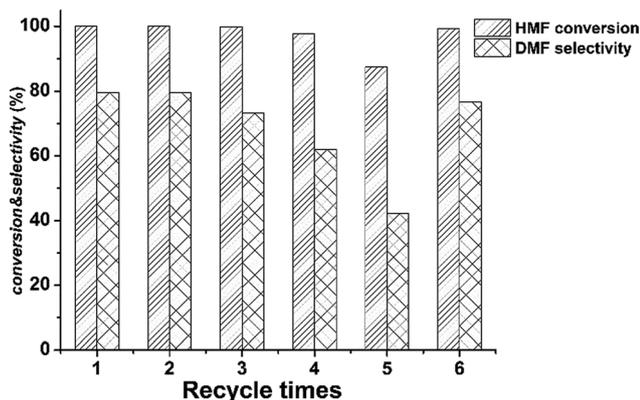
Fig. 4 Reusability of the Ru-MoO<sub>x</sub>/C catalyst. Reaction condition: 180 °C, 1.5 MPa of H<sub>2</sub>, 1 h, HMF 0.5 g, *n*-butyl alcohol 40 ml and 5% Ru-10% MoO<sub>x</sub>/C catalyst 0.1 g.
