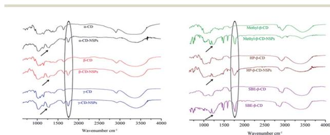
Fig. 2 FTIR spectra of  $\alpha$ ,  $\beta$ ,  $\gamma$ -CD and  $\beta$ -CD derivative NSPs (left) in comparison with their monomers (right) for chemical structural analysis. The specific peaks for carbonyl in the NSP spectra are marked.
