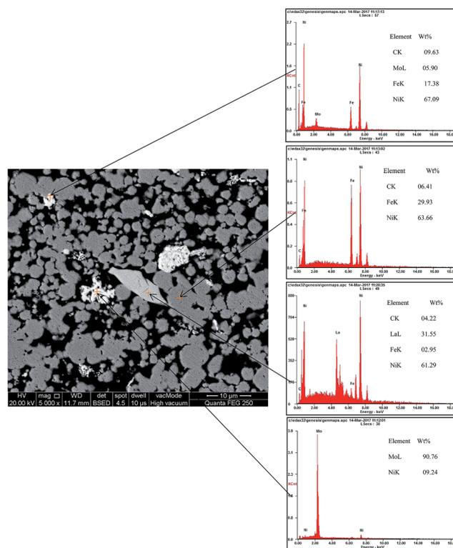
Fig. 3 BSED and EDS of porous Ni–Fe–Mo–C–LaNi<sub>5</sub> electrode.
