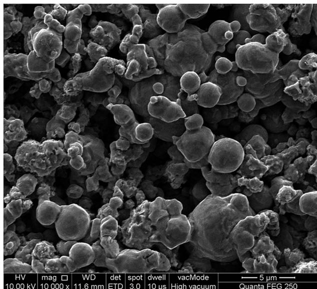
Fig. 2 SEM images of the freshly prepared porous Ni–Fe–Mo–C–LaNi<sub>5</sub> electrode.
