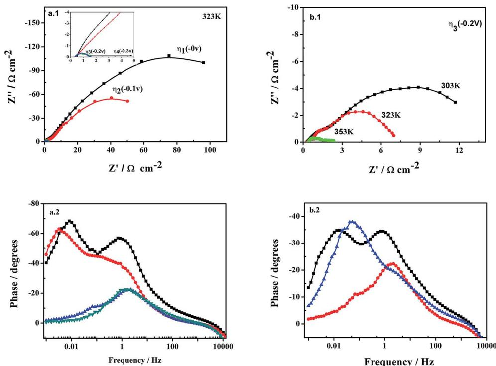
Fig. 8 Impedance data obtained for the porous Ni-Fe-Mo-C/LaNi<sub>5</sub> electrode in 6 M KOH solution at: (a) 323 K (effect of overpotential): (a.1) Nyquist representation, (a.2) Bode representation of the phase angle as a function of frequency; and at overpotential (effect of temperature): (b.1) Nyquist representation, (b.2) Bode representation of the phase angle as a function of frequency.
