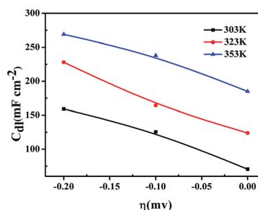
Fig. 10 Trend of the double layer capacitance,  $C_{dl}$ , as a function of the HER overpotential for porous Ni-Fe-Mo-C-LaNi<sub>5</sub> electrode in 6 M KOH solution at: 303 K, 323 K and 353 K.
