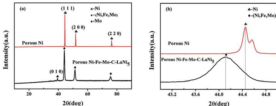
Fig. 1 (a) XRD pattern of the porous Ni–Fe–Mo–C–LaNi<sub>5</sub> cathode material and porous Ni; (b) the negative shift of the (111) peak of the porous Ni–Fe–Mo–C–LaNi<sub>5</sub> cathode material relative to that of the porous Ni.
