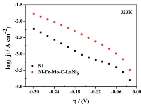
Fig. 7 Linear Tafel polarization curves recorded on smooth Ni, Ni-Fe-Mo-C-LaNi<sub>5</sub> electrocatalysts in 6 M KOH solution at 323 K.
