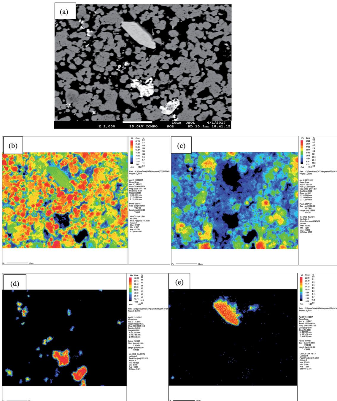
Fig. 4 BSED images (a) and EPMA mappings of porous Ni–Fe–Mo–C–LaNi<sub>5</sub> electrode, showing the elemental distribution of Ni (b), Fe (c), Mo (d) and La (e).
