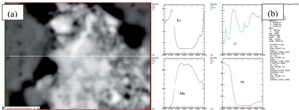
Fig. 5 BSED images (a) and EPMA Line scanning (b) of porous Ni-Fe-Mo-C-LaNi<sub>5</sub> electrode, showing the elemental distribution of Ni, Fe, Mo and C.
