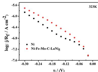
**Fig. 11** Linear Tafel polarization curves recorded on Ni-Fe-Mo-C-LaNi<sub>5</sub> and Ni electrocatalytic in 6 M KOH solution at 323 K, corrected considering the surface roughness factor,  $R_f$ .
