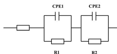
Fig. 9 EEC models used to explain the EIS response of the HER on the Ni-Fe-Mo-C-LaNi<sub>5</sub>; two-time constant serial model (2 TS).
