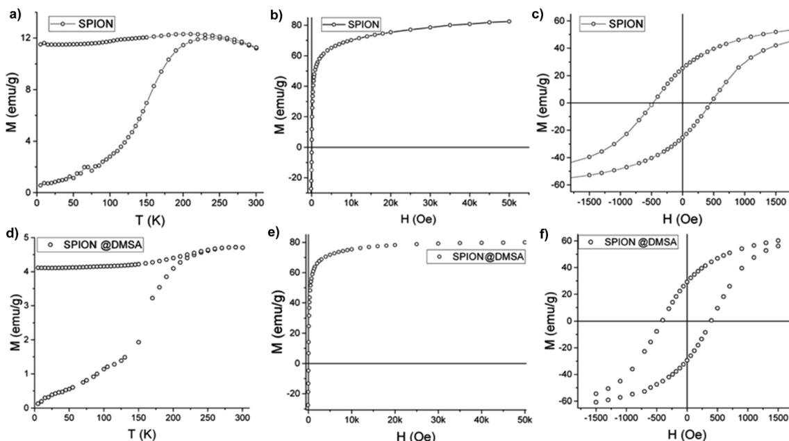
**Fig. 6** Magnetic data on SPION@OA (upper panels) and SPION@DMSA (lower panels): (a and d) ZFC-FC magnetization curves; (b and e) magnetization at 300 K; (c and f) enlargement of the low field region of the hysteresis cycle at 2.5 K.
