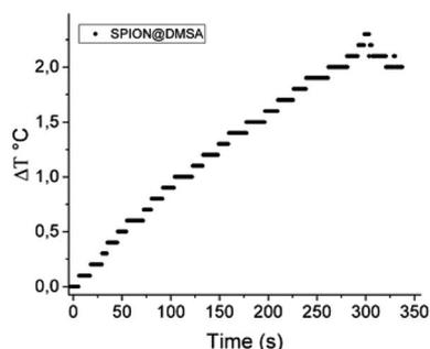
Fig. 7 Temperature kinetics of a water suspension of SPION@DMSA, 0.77 mg mL<sup>-1</sup> Fe, during the exposure to the alternating magnetic field (17.1 kA m<sup>-1</sup>, 183 kHz). The starting temperature was 295 K.
