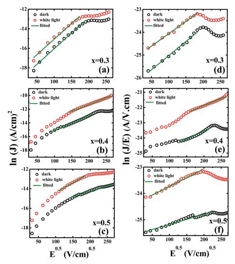
Fig. 9 Leakage current density (J) as function of electric field (E) fitted with Schottky emission (a) x = 0.3, (b) x = 0.4, (c) x = 0.5 and fitted with modified Schottky–Simmons equation/Poole–Frenkel model (d) x = 0.3, (e) x = 0.4, (f) x = 0.5 under dark and illumination of white light.
