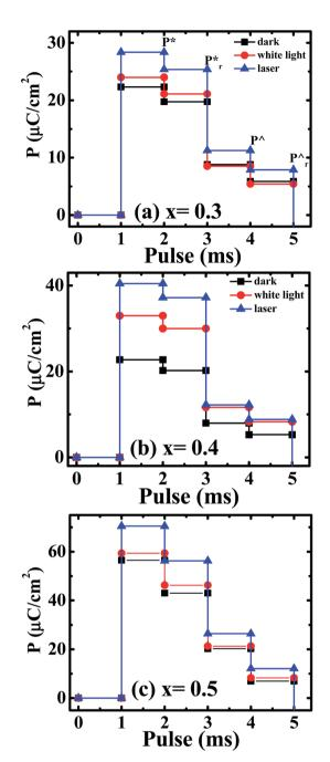
Fig. 7 PUND characteristics for poled ceramics at applied E-field 80 kV cm $^{-1}$  and pulse width 100 ms under dark and illuminated conditions for (a) x = 0.3, (b) x = 0.4, (c) x = 0.5.
