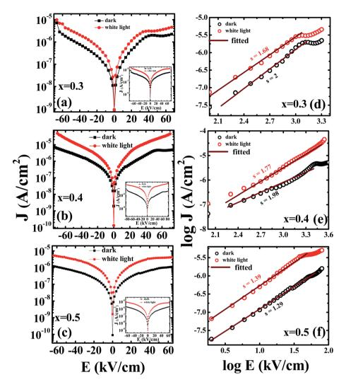
Fig. 8 Leakage current density (J) as function of electric field (E) for PLBZT systems for poled electroceramics (inset unpoled) under dark and illumination of white light source: (a) x = 0.3, (b) x = 0.4, (c) x = 0.5. Conduction mechanisms for PLBZT ceramics studies using J-E characteristics SCLC process for electrically poled electroceramics and fitted with SCLC (log(J) vs. log(E)) plots for (d) x = 0.3, (e) x = 0.4, (f) x = 0.5.
