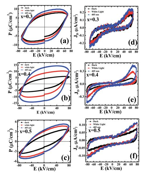
Fig. 6 Ferroelectric polarization measured under three different condition *i.e.* dark, white light source and monochromatic laser having 405 nm wavelength for x = 0.3 (a), 0.4 (b), 0.5 (c). Switching of displacement current derived from ferroelectric polarization loop for x = 0.3 (d), 0.4 (e), 0.5 (f).
