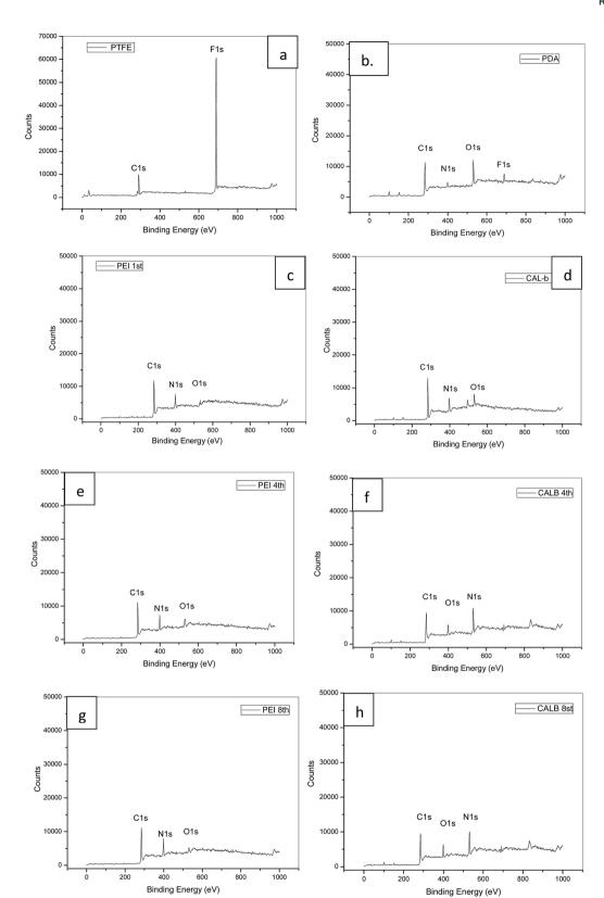
Fig. 5 (a-h) XPS spectra for PTFE, PDA-modified PTFE, PEI and lipase deposited PTFE membranes
