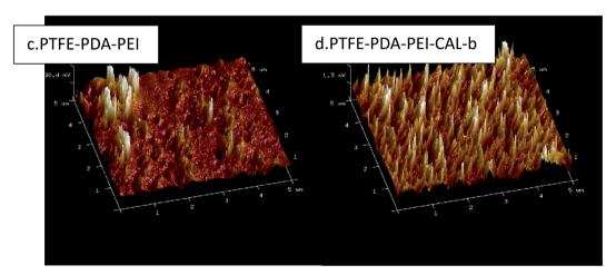
Fig. 7 (a-d) AFM photographs of modified and unmodified PTFE surface.
