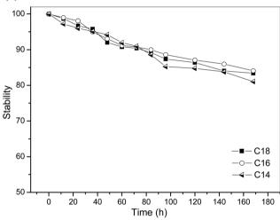
Fig. 8 (a) Conversion rate of different oleates under the same reaction conditions. Setup: molar ratio: 1:1, length of microreactor: 5 m, temperature: 40 °C, reaction time: 25 min. (b) Reusability of microreactor on esterification of oleate. Setup: molar ratio: 1:1, length of microreactor: 5 m, temperature: 40 °C, reaction time: 25 min.
