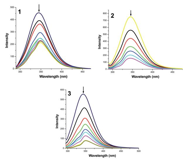
Fig. 9 The emission spectrum of BSA (1  $\mu$ M;  $\lambda_{exc}$  = 280 nm;  $\lambda_{emi}$  = 345 nm) in the presence of increasing amounts of the complexes 1–3 (0–35  $\mu$ M). The arrow shows the fluorescence quenching upon increasing complex concentration.
