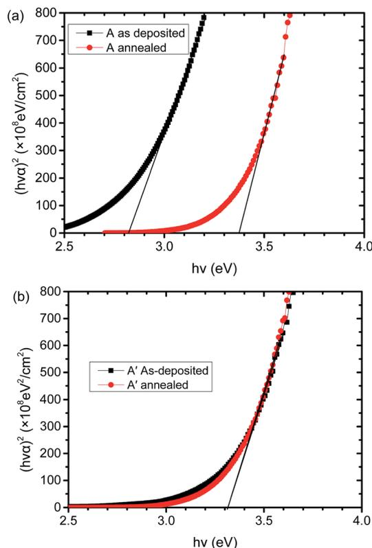
**Fig. 4** Relation between  $(h\nu\alpha)^2$  and  $(h\nu)$ : (a) sample A (deposited in an Ar/O<sub>2</sub> atmosphere at 388 nm at an annealing temperature of 620 °C); (b) sample A' (deposited in an Ar atmosphere at 627 nm at an annealing temperature of 620 °C).
