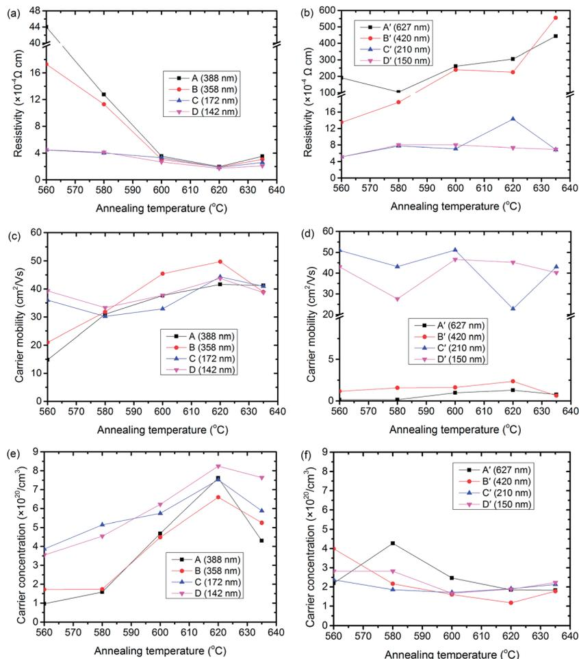
Fig. 2 Properties of annealed samples: (a) resistivity of Ar/O<sub>2</sub> atmosphere deposited films; (b) resistivity of Ar atmosphere deposited films; (c) carrier mobility of Ar/O<sub>2</sub> atmosphere deposited films; (d) carrier mobility of Ar atmosphere deposited films; (e) carrier concentration of Ar/O<sub>2</sub> atmosphere deposited films; (f) carrier concentration of Ar atmosphere deposited films.
