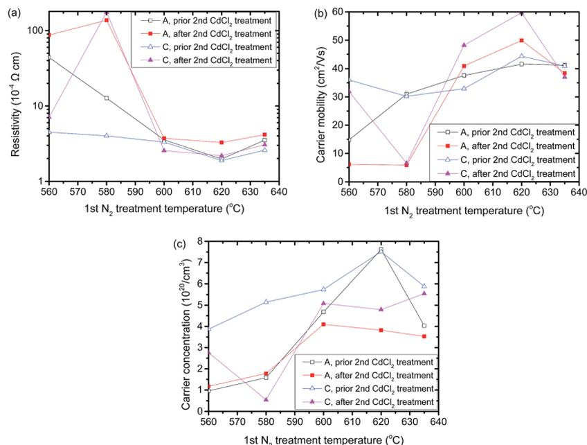
**Fig. 5** Electrical properties of N<sub>2</sub> gas annealed samples A and C before and after chloride treatment, where (a) is the resistivity, (b) is the carrier mobility and (c) is the carrier concentration.
