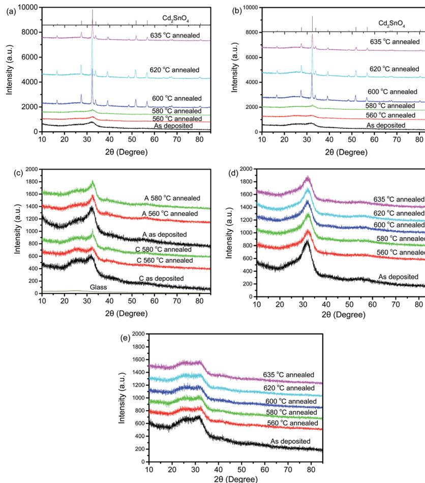
**Fig. 1** XRD patterns of some samples: (a) sample A (Ar/O<sub>2</sub> atmosphere deposited, 388 nm), (b) sample C (Ar/O<sub>2</sub> atmosphere deposited, 172 nm), (c) low temperature annealed samples A and C, (d) sample A' (Ar atmosphere deposited, 627 nm) and (e) sample C' (Ar atmosphere deposited, 210 nm).
