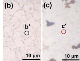
Fig. 56 (a) Low-magnification optical microscope image of as-synthesized graphene on Ni/SiO<sub>2</sub>/Si substrate using 2 sccm CH<sub>4</sub>, 30 s growth duration and a fast cooling process. (b) & (c) High-magnification images of the regions corresponding to the region in (a). Dashed circle in (a) presents a boundary where graphene is synthesized. This figure has been adapted/reproduced from ref. 179 with permission from Springer.
