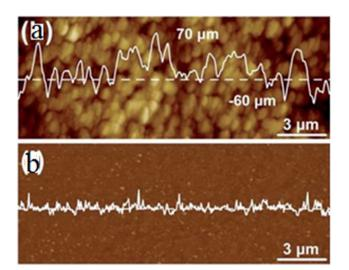
Fig. 57 (a) AFM image of Ni/Mo substrate after annealing at  $1000\,^{\circ}\text{C}$ , (b) AFM image of graphene transferred onto  $\text{SiO}_2/\text{Si}$  substrate. Insets are line profiles at the dashed line. This figure has been adapted/reproduced from ref. 179 with permission from Springer.
