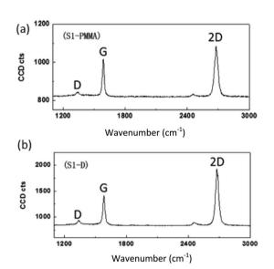
Fig. 23 Raman spectra (532 nm laser excitation wavelength) for graphene transferred onto the  $\rm SiO_2$ -on-Si substrate. (a) Raman spectra obtained from a sample prepared by the standard PMMA-based method. (b) Raman spectra obtained from a sample obtained by the direct transfer method. This figure has been adapted/reproduced from ref. 123 with permission from World Scientific.
