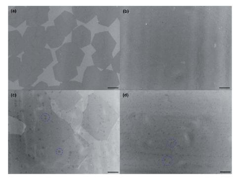
Fig. 42 SEM images of CVD graphene on Cu: (a) 5 ppm  $CH_4$  for 60 min, (b) 10 ppm  $CH_4$  for 60 min, (c) 20 ppm  $CH_4$  for 30 min, (d) 30 ppm  $CH_4$  for 20 min. Some are highlighted by dashed blue circles in images (c) and (d) and represent multilayer graphene domains. This figure has been adapted/reproduced from ref. 153 with permission from Institute of Physics Publishing.
