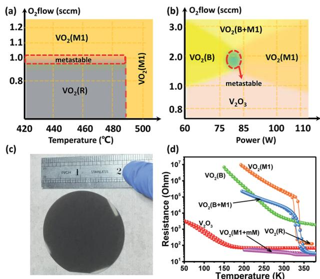
Fig. 4 Phase diagram for different polymorphs of vanadium oxide thin films with growth temperature and oxygen flow (a), and RF power and oxygen flow (b). (c) The wafer scale production of  $VO_2$  epitaxial polymorphs in M1 phase. (d) Transport properties of different epitaxial polymorphs of  $VO_2$  and  $V_2O_5$  epitaxial thin films.
