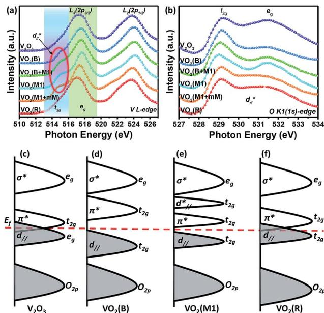
Fig. 5 X-ray absorption spectroscopy (XAS) of V L (a) and O K (b) edges in the various epitaxial vanadium oxide polymorphs. Diagrams illustrate the electronic structures of  $V_2O_3$  in (c),  $VO_2$  (B) in (d),  $VO_2$  (M1) in (e), and  $VO_2$  (R) in (f) in terms of Goodenough's rules.
