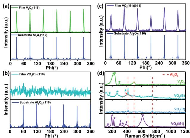
Fig. 2 Phi scans of different vanadium oxide epitaxial thin films. (a)  $V_2O_3$ . (b)  $VO_2$  (M1), and (c)  $VO_2$  (B). (d) Raman spectra of different epitaxial polymorphs of  $VO_2$  and  $V_2O_3$  thin films. The Raman peaks at around 417, 499, and 749  $cm^{-1}$  (marked by the dashed red lines) are assigned to the  $Al_2O_3$  substrate.
