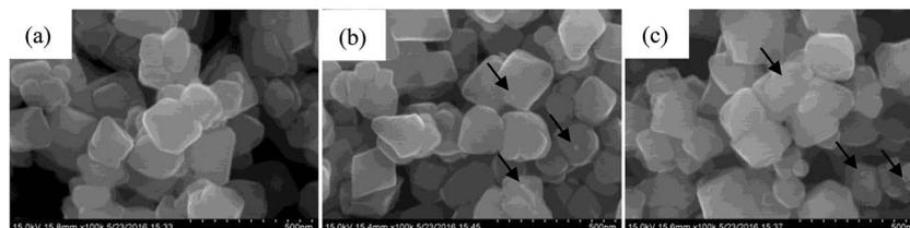
Fig. 2 The SEM images of  $\text{Fe}_3\text{O}_4$  (a),  $\text{Fe}_3\text{O}_4@NH_2Q$  (b) and  $\text{Fe}_3\text{O}_4@COOHQ$  (c).
