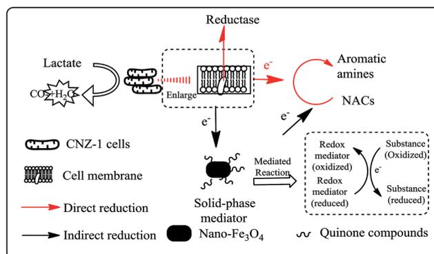
Fig. 9 The proposed mechanism of Fe<sub>3</sub>O<sub>4</sub>@COOHQ mediated NACs reduction by strain CNZ-1.
