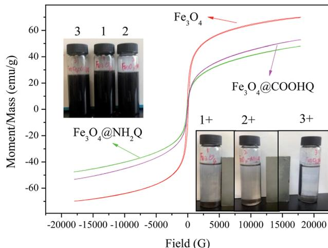
Fig. 6 VSM analyses of  $\text{Fe}_3\text{O}_4@NH_2Q$  and  $\text{Fe}_3\text{O}_4@COOHQ$ .
