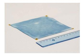
Fig. 10 Picture of (13 cm  $\times$  13 cm) PET fabric covered by PRAP-CVD PEDOT film.
