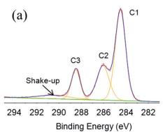
Fig. 7 XPS C 1s high resolution spectra of (a) PET and (b) PEDOT/PET and relatively chemical states.
