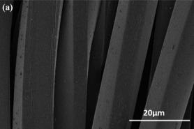
Fig. 9 SEM images of PEDOT/PET at (a) strain of 175% before unloading and (b) relaxed state after unloading corresponding to a strain of 100%.
