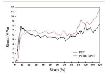
Fig. 8 Typical stress vs. strain curves of untreated PET fabric and PEDOT/PET fabric at  $0.0025~\rm s^{-1}$  and  $20~\rm ^{\circ}C$ .
