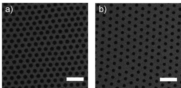
Fig. 2 Scanning electron micrographs of polyNIPAM colloids deposited onto glass substrates at different temperatures using dip coating: (a) deposition at  $20 \text{ }^\circ\text{C}$  and (b) deposition at  $50 \text{ }^\circ\text{C}$ . Scale bar:  $5 \mu\text{m}$ .
