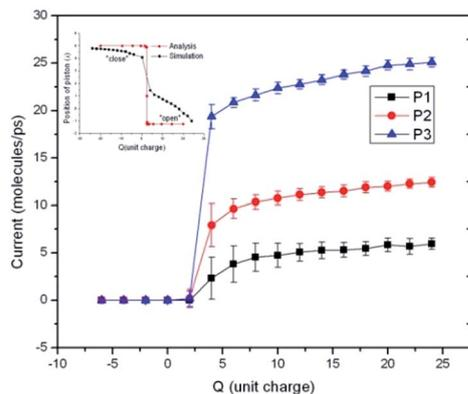
Fig. 2 Charge dependence of the water flux in carbon nanotubes for different water pressure gradients. The pressure gradients of  $P_1$ ,  $P_2$  and  $P_3$  is  $2 \times 10^7$ ,  $4 \times 10^7$  and  $1 \times 10^8$  Pa  $\text{\AA}^{-1}$  respectively.
