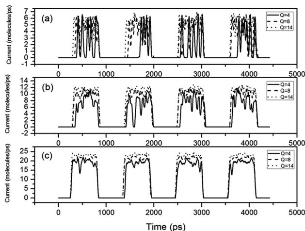
Fig. 4 Water currents change with time under different pressure gradients. The pressure gradients are (a)  $2 \times 10^7$ , (b)  $4 \times 10^7$  and (c)  $1 \times 10^8$  Pa  $\text{\AA}^{-1}$ , respectively.
