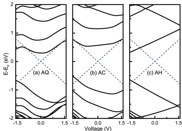
Fig. 3 Evolution of MPSH eigenvalues under bias voltages for (a) AQ, (b) AC, and (c) AH. The dashed blue lines indicate the bias window.
