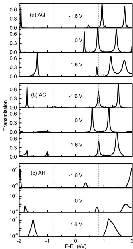
Fig. 5 Electronic transmission spectra for (a) AQ, (b) AC and (c) AH at  $-1.6$ ,  $0$ ,  $1.6$  V. The dashed blue lines indicate the bias window.
