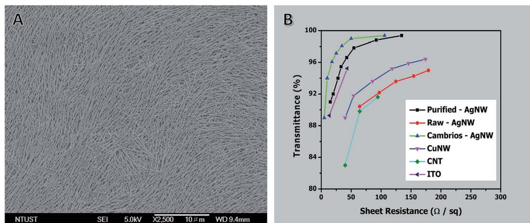
Fig. 8 (A) Typical FE-SEM image of AgNW film. (B) A plot of specular transmittance ( $\lambda = 550 \text{ nm}$ ) versus sheet resistance for AgNW films before and after purification. Each data point is the average of five measurements. The performances of AgNWs,<sup>42</sup> CuNWs,<sup>94</sup> CNT,<sup>95</sup> and ITO are shown for comparison.
