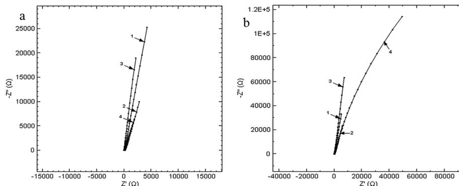
Fig. 6 Nyquist diagrams at immersion (a) and after keeping the Ti10Zr for 24 hours (b), in the 4 media, on the frequency range  $0.1 \div 10^5$  Hz I<sub>a</sub> PCD: (1) CL, (2) CH, (3) SF and (4) RAS.
