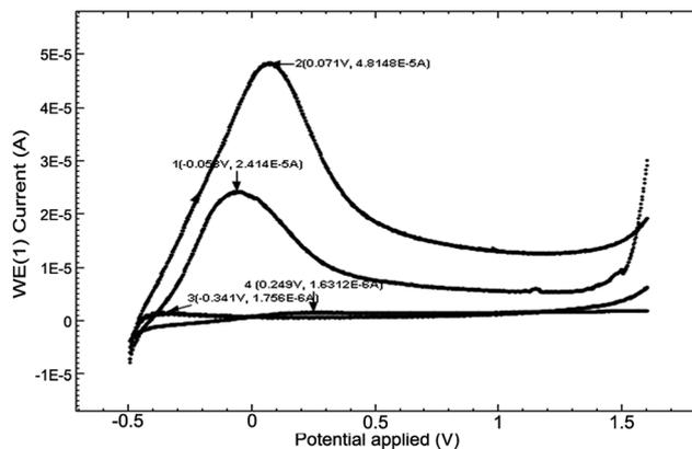
**Fig. 4** Linear voltammetry (LV) for the 4 media, at scanning speeds of  $50 \text{ mV s}^{-1}$ , at 24 hours following the immersion: (1) CL, (2) CH, (3) SF and (4) RAS of alloy Ti10Zr.
