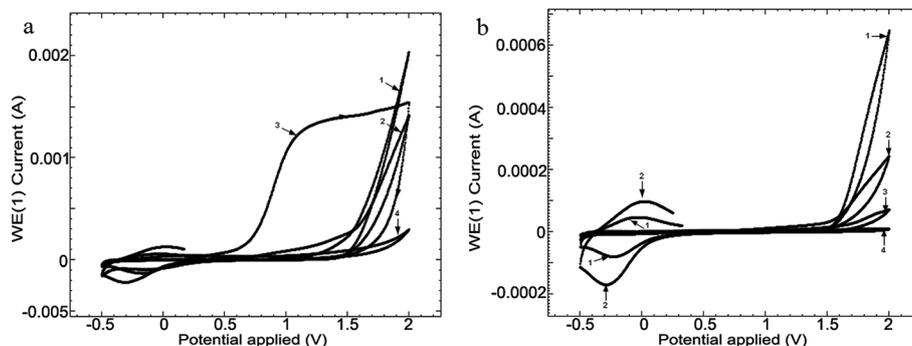
**Fig. 3** Cyclic voltammograms (CV) obtained in the 4 media when immersing Ti10Zr (a) and after 24 hours after immersion (b): CL (1), CH (2), SF (3) and RAS (4), at a scanning speed of  $100 \text{ mV s}^{-1}$ . The pitting corrosion of Ti10Zr immersed in the 4 media shows up only in SF at high potentials, in the field: 2.73–3.00 V.
