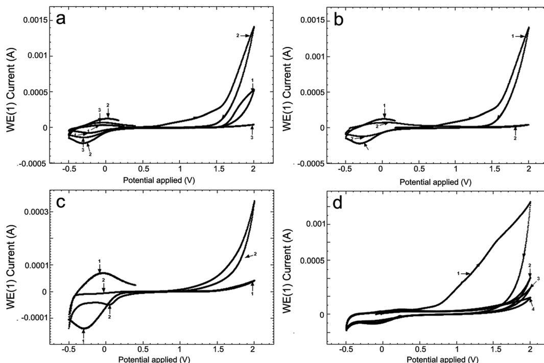
Fig. 2 Cyclic voltammograms (CV) for (a) Ti10Zr alloy at  $100\text{ mV s}^{-1}$  in (1) CL, (2) CH, (3) acetate lock (AL); (b) Ti10Zr in ChitHigh immediately after immersion (1) and 4 days after immersion (2); (c) in acetate lock on Ti10Zr (1) and on Pt (2); (d) in acid medium ( $\text{pH} = 1.00$ ) at different moments after immersion: (1) immediately after immersion, (2) at 5 minutes after immersion, (3) at 80 minutes after immersion, (4) at 17 hours after immersion.
