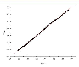
Fig. 5 Plot of  $\gamma_{\rm est}$  vs.  $\gamma_{\rm exp}$  for the [C<sub>n</sub>mim][TFA] ILs.  $\gamma_{\rm est}=1.01439\gamma_{\rm exp}-0.6287; r=0.999, s=0.1059.$
