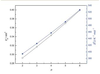
Fig. 3 Plots of  $V_{\rm m}$  (298.15 K) vs. number of carbons (n) in the alkyl chains of the ILs and  $S^0$  (298.15 K) vs. n. ( $\blacksquare$ :  $V_m = 0.23786 + 0.02665n$ , and r = 0.999).
