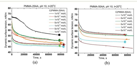
Fig. 3 Dynamic surface tension of aqueous polymer solutions vs. time for different polymer concentrations (a) PMMA–25AA,  $C_p = 1 \times 10^{-7}$  to 1  $\times$  10<sup>-4</sup> mol L<sup>-1</sup>; (b) PMMA–50AA,  $C_p = 1 \times 10^{-6}$  to 5  $\times$  10<sup>-4</sup> mol L<sup>-1</sup>. Temperature is 20 °C; pH = 10.
