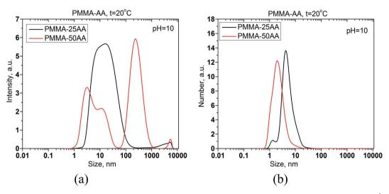
Fig. 2 Mean size distribution by intensity (a) and by number (b) for PMMA-25AA and PMMA-50AA at concentrations of  $1 \times 10^{-4}$  mol L $^{-1}$  and  $5 \times 10^{-4}$  mol L $^{-1}$ , correspondingly. Temperature is 20 °C, pH = 10.
