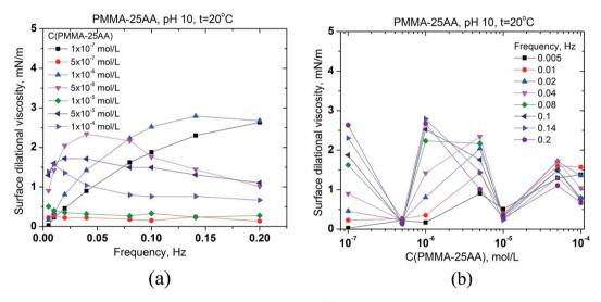
Fig. 7 Surface dilational viscosity of aqueous solutions of PMMA–25AA (a) vs. the frequency of oscillation of the air bubble for different copolymer concentrations in the range  $1\times10^{-7}$  to  $1\times10^{-4}$  mol L<sup>-1</sup>; (b) vs. the copolymer concentration for different oscillation frequencies in the range of 0.005–0.2 Hz. Temperature is 20 °C, pH = 10.
