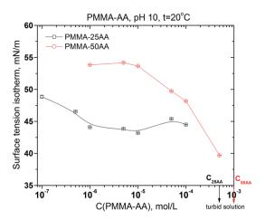
Fig. 4 Equilibrium surface tension of aqueous solutions of PMMA–25AA and PMMA–50AA vs. concentration. Temperature is 20  $^{\circ}$ C; pH = 10
