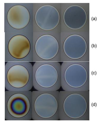
Fig. 10 Characteristic snapshots illustrating the time evolution of microscopic foam films from aqueous solutions of PMMA–50AA for different polymer concentration. Temperature is 20 °C, pH = 10, the film radius is 100  $\mu m$ . (a)  $1\times 10^{-6}$  mol L $^{-1}$ : 11.44 s, 34.57 s, 5.24 min; (b)  $5\times 10^{-6}$  mol L $^{-1}$ : 14.56 s, 36.16 s, 5.19 min; (c)  $1\times 10^{-5}$  mol L $^{-1}$ : 12.56 s, 37.52 s, 5.08 min; (d)  $5\times 10^{-5}$  mol L $^{-1}$ : 13.46 s, 43.44 s, 5.09 min.
