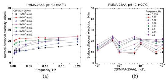
Fig. 5 Surface dilational elasticity of aqueous solutions of PMMA-25AA (a) vs. the frequency of oscillation of the air bubble for different polymer concentrations in the range  $1 \times 10^{-7}$  to  $1 \times 10^{-4}$  mol L<sup>-1</sup>; (b) vs. the polymer concentration for different oscillation frequencies in the range of 0.005-0.2 Hz. Temperature is 20 °C, pH = 10.
