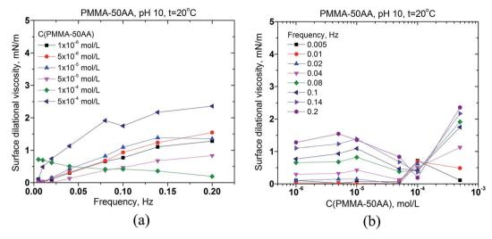
Fig. 8 Surface dilational viscosity of aqueous solutions of PMMA-50AA (a) vs. the frequency of oscillation of the air bubble for different copolymer concentrations in the range  $1 \times 10^{-6}$  to  $5 \times 10^{-4}$  mol L<sup>-1</sup>; (b) vs. the copolymer concentration for different oscillation frequencies in the range of 0.005-0.2 Hz. Temperature is 20 °C, pH = 10.
