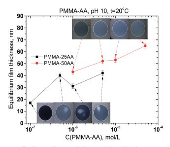
**Fig. 12** Equilibrium thickness of microscopic foam films from aqueous solutions of PMMA–25AA and PMMA–50AA *versus* polymer concentration. Temperature is 20 °C, pH = 10, the film radius is 100  $\mu$ m. Insets: characteristic snapshots of the films at  $\sim\!\!5$  min after their formation.
