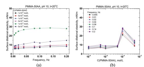
Fig. 6 Surface dilational elasticity of aqueous solutions of PMMA–50AA (a) vs. the frequency of oscillation of the air bubble for different polymer concentrations in the range  $1 \times 10^{-6}$  to  $5 \times 10^{-4}$  mol L<sup>-1</sup>; (b) vs. the polymer concentration for different oscillation frequencies in the range of 0.005–0.2 Hz. Temperature is 20 °C, pH = 10.
