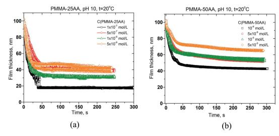
Fig. 11 Time evolution of the mean thickness of foam films from aqueous solutions of (a) PMMA-25AA, and (b) PMMA-50AA, for various polymer concentrations. Temperature is 20 °C; pH = 10; the film radius is 100  $\mu$ m.
