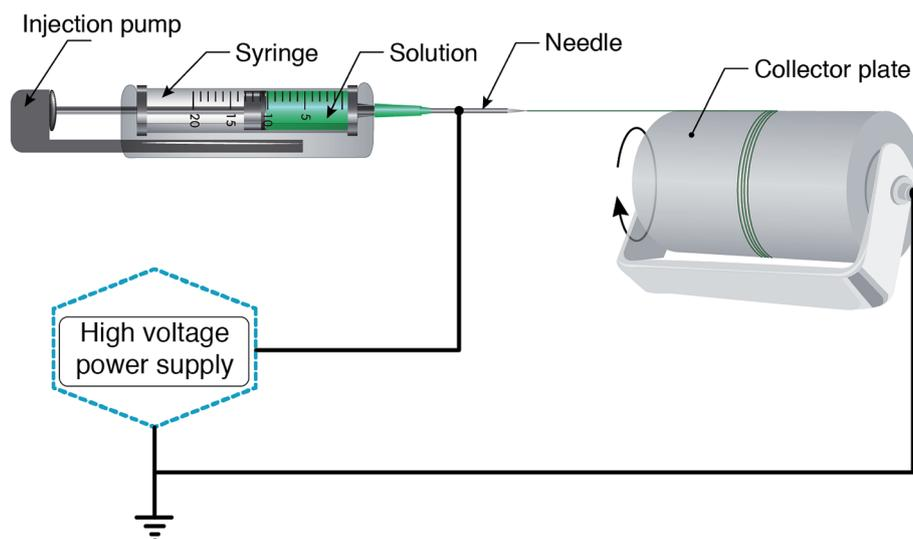
Fig. 2 Schematic of a typical setup for electrospinning.
