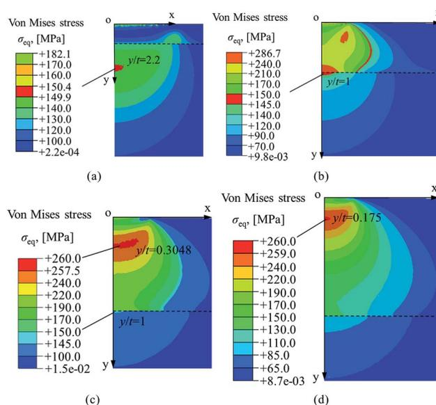
Fig. 7 Typical locations of yield inception in cylindrical coating/substrate composites under (a)  $E_{co} = 250$  GPa,  $Y_{co} = 260$  MPa,  $t/R = 0.001$ ; (b)  $E_{co} = 391$  GPa,  $Y_{co} = 638$  MPa,  $t/R = 0.005$ ; (c)  $E_{co} = 250$  GPa,  $Y_{co} = 260$  MPa,  $t/R = 0.0105$ ; and (d)  $E_{co} = 250$  GPa,  $Y_{co} = 260$  MPa,  $t/R = 0.016$ .
