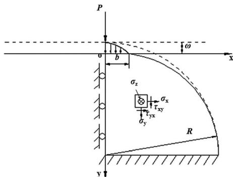
Fig. 2 Hertz contact between a cylindrical coating and a rigid plane.
