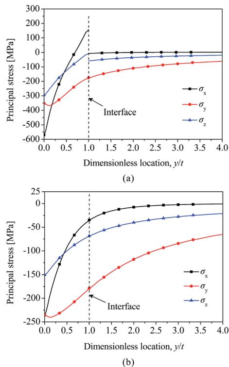
Fig. 8 Principal stresses along the axis of symmetry of cylinders with coating properties of (a)  $E_{co} = 448$  GPa,  $Y_{co} = 836$  MPa and (b)  $E_{co} = 130$  GPa,  $Y_{co} = 150$  MPa under the substrate parameters of  $E_{su} = 130$  GPa,  $Y_{su} = 150$  MPa at  $t/R = 0.003$ .
