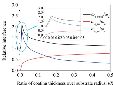
Fig. 9 Critical interference of the coated cylinder relative to the value of a homogeneous one at the yielding inception and the corresponding components with the increasing ratio of coating thickness over substrate radius.
