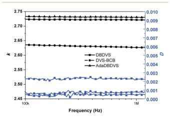
Fig. 9 Frequency dependency of the dielectric constant and dielectric loss of the polymers at room temperature.
