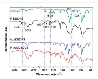
Fig. 5 FTIR spectra of the cured resins compared with that of their corresponding monomers.
