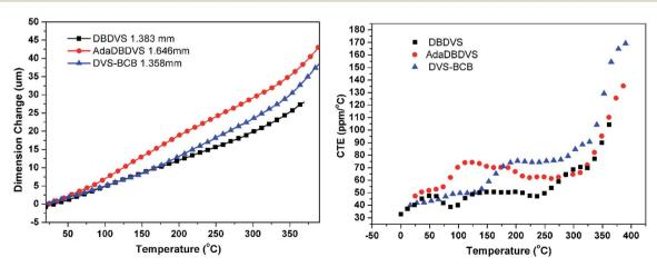
Fig. 8 TMA curves of the cured polymers (left) and CTE versus temperature (right).
