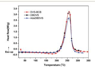
Fig. 4 DSC curves of DBDVS and AdaDBDVS.
