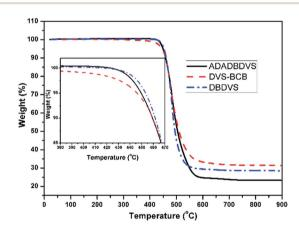
Fig. 6 TGA curves of cured DVS-BCB, DBDVS and AdaDBDVS
