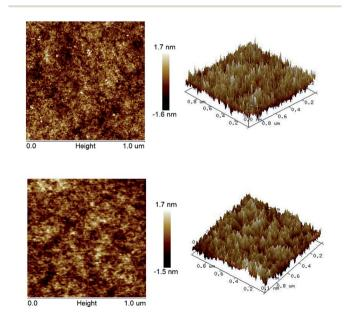
Fig. 10 AFM images of polymeric coatings on a silicon wafer: p-DBDVS (up) and p-AdaDBDVS (bottom); (left) planar graph, (right) stereogram.
