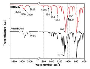
Fig. 3 FTIR spectra of DBDVS and AdaDBDVS monomers.
