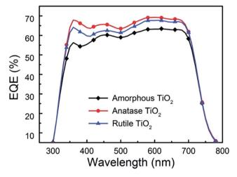
Fig. 7 The IPCE spectra of inverted devices using amorphous, anatase and rutile  $TiO_2$  as electron extraction layers.
