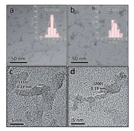
Fig. 1 TEM images of anatase (a) and rutile (b) TiO<sub>2</sub> nanocrystals. HRTEM image of anatase (c) and rutile (d) TiO<sub>2</sub> nanocrystals.
