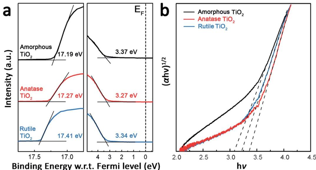
Fig. 4 (a) UPS spectra of various TiO<sub>2</sub> (amorphous, anatase and rutile TiO<sub>2</sub>) films on ITO. (b) The plots of  $(\alpha hv)^{1/2}$  versus photon energy ( $h\nu$ ) for the three types of TiO<sub>2</sub> films prepared on the quartz substrates.
