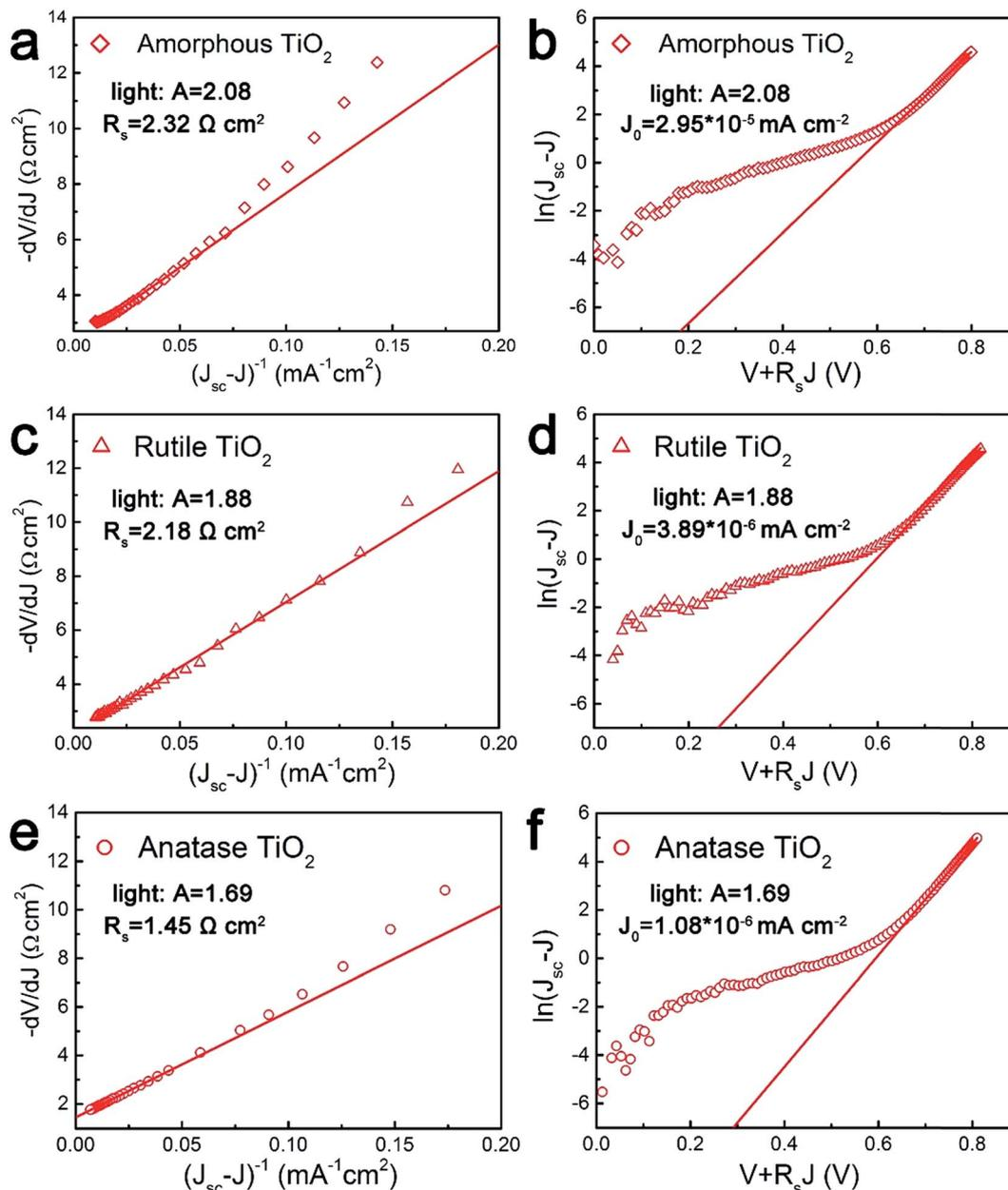
Fig. 9 Plots of  $-dV/dJ$  vs.  $(J_{sc} - J)^{-1}$  and the linear fitting curves (a), (c) and (e), plots of  $\ln(J_{sc} - J)$  against  $V + R_s J$  and the linear fitting curves (b), (d) and (f) from the devices fabricated by using amorphous, rutile and anatase  $\text{TiO}_2$  as electron extraction layers.
