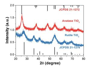
Fig. 2  $\,$  XRD patterns of anatase and rutile  $\,$ TiO $_{2}$  nanocrystals.
