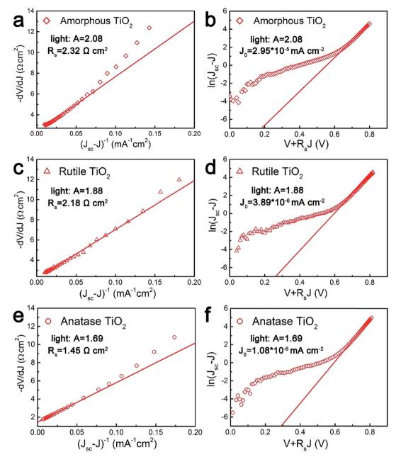
Fig. 9 Plots of -dV/dJ vs.  $(J_{SC} - J)^{-1}$  and the linear fitting curves (a), (c) and (e), plots of  $\ln(J_{SC} - J)$  against  $V + R_S J$  and the linear fitting curves (b), (d) and (f) from the devices fabricated by using amorphous, rutile and anatase  $TiO_2$  as electron extraction layers.
