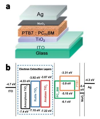
Fig. 5 (a) The structure of the inverted polymer solar cells. (b) Energy level diagram of the component materials used in device fabrication.
