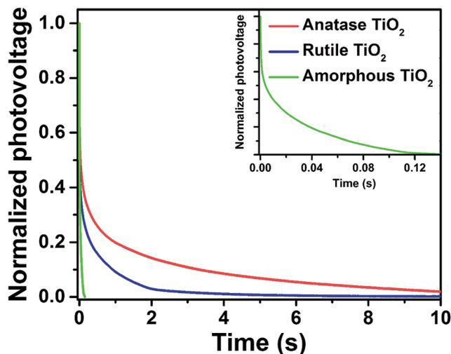
Fig. 10 Open-circuit voltage decays for the three types of TiO<sub>2</sub> based OSCs.
