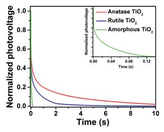
Fig. 10 Open-circuit voltage decays for the three types of  ${\rm TiO_2}$  based OSCs.
