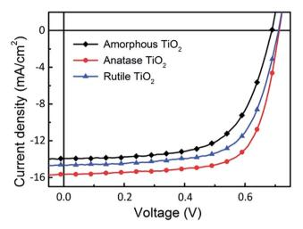
Fig. 6 The J-V characteristics of the inverted devices using amorphous, anatase and rutile  $TiO_2$  as electron extraction layers.
