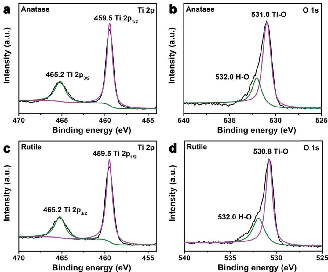
Fig. 3 XPS spectra of anatase and rutile  $\text{TiO}_2$  nanocrystals. High resolution Ti 2p spectra for (a) anatase and (c) rutile  $\text{TiO}_2$  nanocrystals. High resolution O 1s spectra for (b) anatase and (d) rutile  $\text{TiO}_2$  nanocrystals.
