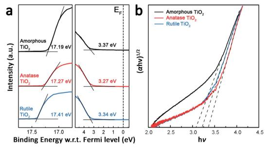
Fig. 4 (a) UPS spectra of various  $TiO_2$  (amorphous, anatase and rutile  $TiO_2$ ) films on ITO. (b) The plots of  $(\alpha h v)^{1/2}$  versus photon energy (hv) for the three types of  $TiO_2$  films prepared on the quartz substrates.
