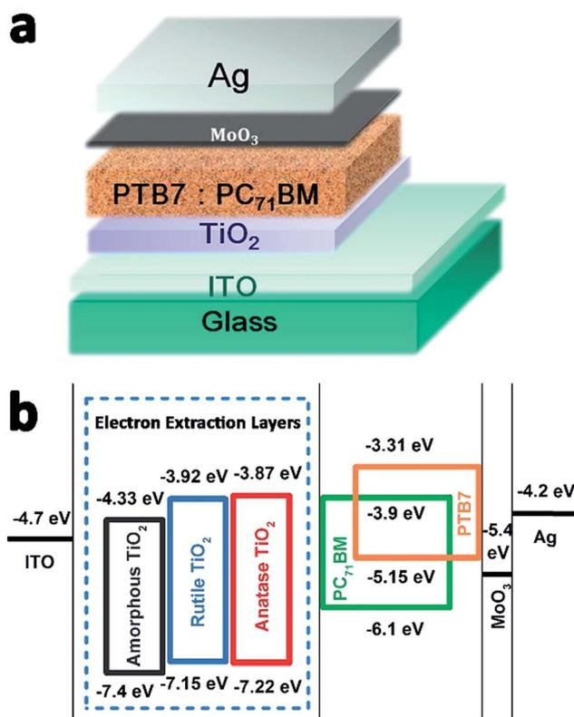
Fig. 5 (a) The structure of the inverted polymer solar cells. (b) Energy level diagram of the component materials used in device fabrication.
