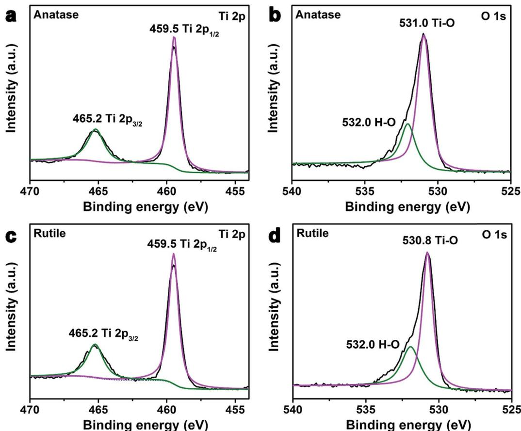
Fig. 3 XPS spectra of anatase and rutile TiO<sub>2</sub> nanocrystals. High resolution Ti 2p spectra for (a) anatase and (c) rutile TiO<sub>2</sub> nanocrystals. High resolution O 1s spectra for (b) anatase and (d) rutile TiO<sub>2</sub> nanocrystals.
