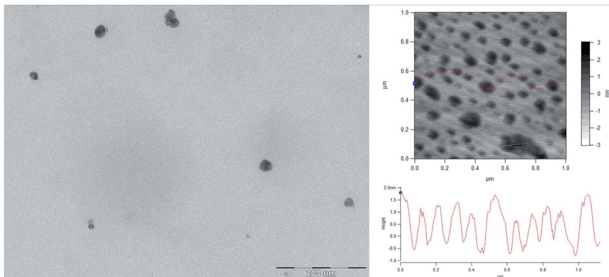
Fig. 5 TEM and AFM with high profile of ground, aq. dispersed and sonicated NaOH-activated PAC (900 °C, 30 min, impregnation ratio 2).
