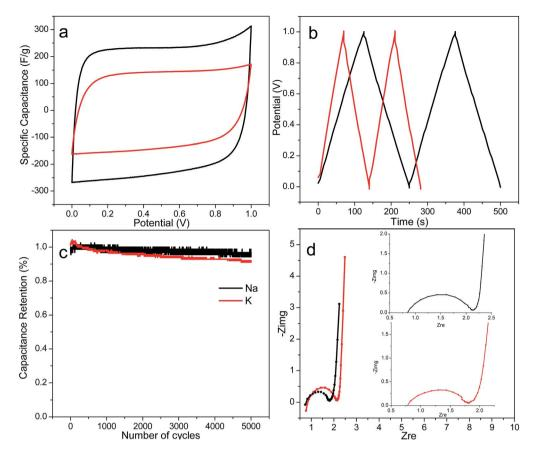
Fig. 6 (a) Cyclic voltagramms at 20 mV s<sup>-1</sup>, (b) galvanostatic charge/discharge curves at 1 A g<sup>-1</sup>, (c) capacitance retention over 5000 cycles under 1 A g<sup>-1</sup>, and (d) Nyquist plots of NaOH and KOH-activated PACs based supercapacitors.
