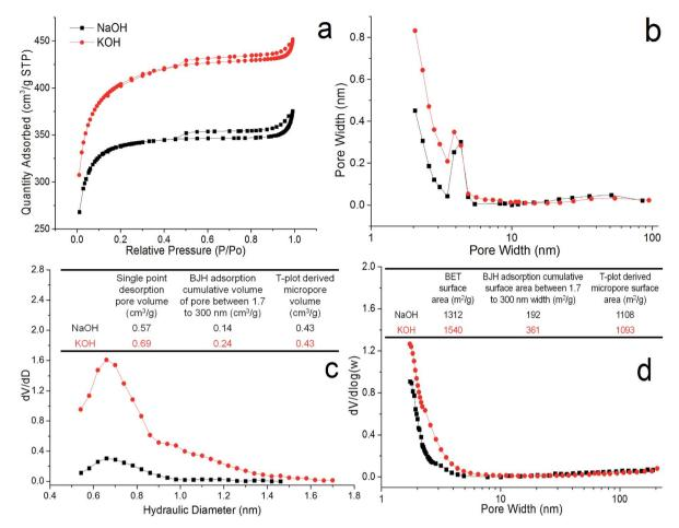
Fig. 3 PACs porous structures (900 °C, ratio 1, 30 min, N<sub>2</sub>): (a) nitrogen adsorption-desorption isotherm; (b) BJH neck size distribution; (c) micropore hydraulic diameter distribution; (d) BJH mesopore/cavity width distribution. Inset tables: (c) pore volume; (d) surface area.
