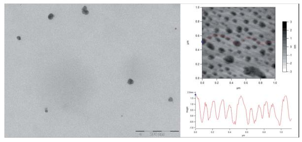
Fig. 5 TEM and AFM with high profile of ground, ag. dispersed and sonicated NaOH-activated PAC (900 °C, 30 min, impregnation ratio 2).
