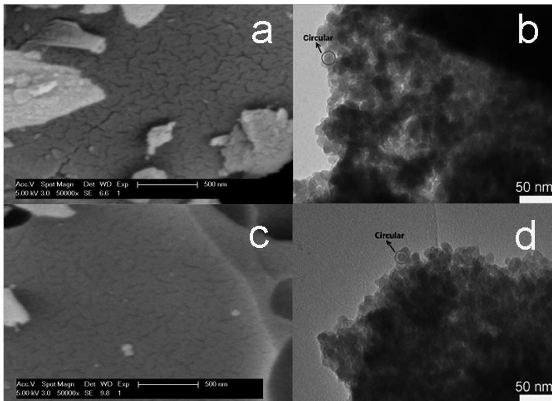
Fig. 4 SEM (a and c) and TEM (b and d) of PACs activated by (a and b) NaOH and (c and d) KOH (900 °C, 30 min, impregnation ratio of 2, N<sub>2</sub>, 10 °C min).
