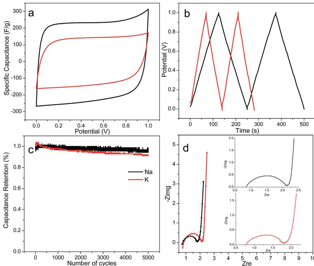
Fig. 6 (a) Cyclic voltammograms at  $20 \text{ mV s}^{-1}$ , (b) galvanostatic charge/discharge curves at  $1 \text{ A g}^{-1}$ , (c) capacitance retention over 5000 cycles under  $1 \text{ A g}^{-1}$ , and (d) Nyquist plots of NaOH and KOH-activated PACs based supercapacitors.
