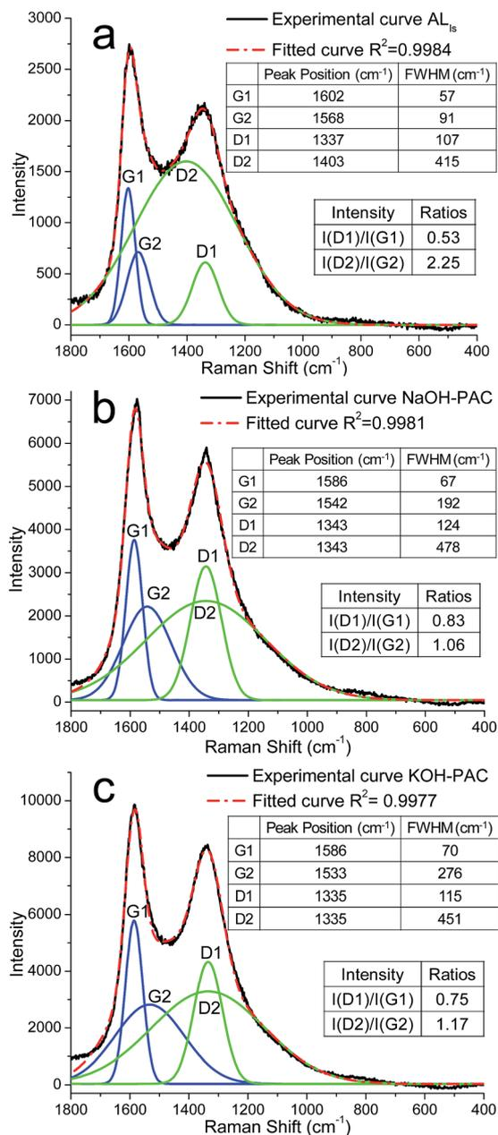
Fig. 2 Raman spectrum of (a) AL<sub>1s</sub> char (b) NaOH and (c) KOH-activated PAC (900 °C, 30 min, N<sub>2</sub>, 10 °C min, ratio 1).
