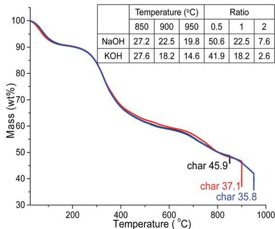
Fig. 1 TGA of  $\text{AL}_{1\text{s}}$  heat to 850, 900 and 950 °C and held for 30 min ( $\text{N}_2$ , 10 °C min). Inset table: yields (wt%) of PACs heated to 850, 900 and 950 °C and held for 30 min (1 impregnation ratio) and activated at 0.5, 1 and 2 alkali hydroxide/ $\text{AL}_{1\text{s}}$  impregnation ratios (900 °C, 30 min).
