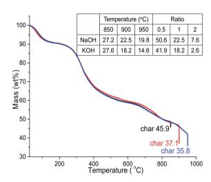
Fig. 1 TGA of  $AL_{ls}$  heat to 850, 900 and 950 °C and held for 30 min  $(N_2, 10$  °C min). Inserted table: yields (wt%) of PACs heated to 850, 900 and 950 °C and held for 30 min (1 impregnation ratio) and activated at 0.5, 1 and 2 alkali hydroxide/ $AL_{ls}$  impregnation ratios (900 °C, 30 min).
