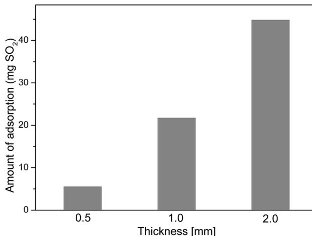
Fig. 6 Effect of the thickness of the MnO<sub>2</sub> filter on the amount of SO<sub>2</sub> adsorption.
