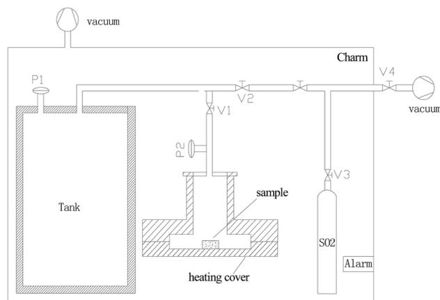
Fig. 2 Schematic diagram of the volumetric test-rig.
