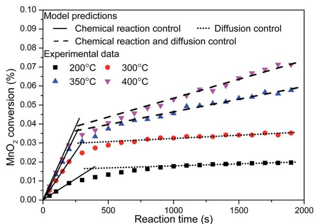
Fig. 10 Experimental data and model predictions of MnO<sub>2</sub> conversion under four reaction temperature conditions.
