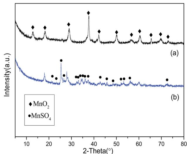
Fig. 4 XRD patterns of MnO<sub>2</sub> filter (a) before and (b) after desulfurization.
