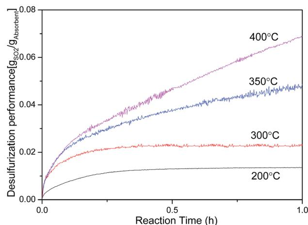
Fig. 5 Influence of temperature on SO<sub>2</sub> capture performance of MnO<sub>2</sub> filter at 200 °C, 300 °C, 350 °C and 400 °C.
