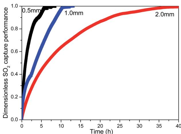
Fig. 7 Effect of the thickness of the MnO<sub>2</sub> filter on the SO<sub>2</sub> adsorption performance.
