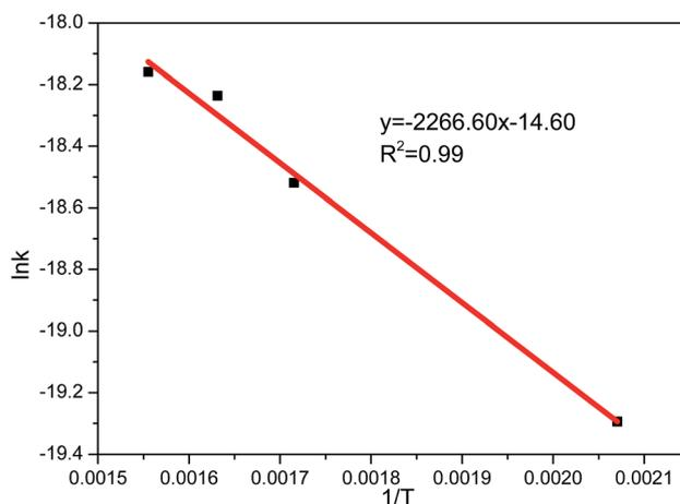
Fig. 11 Arrhenius plot of sulfate rate of MnO<sub>2</sub> filter with chemical reaction control.
