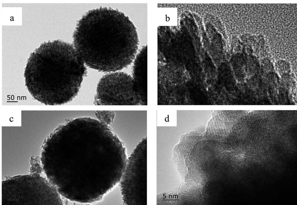
Fig. 9 TEM images of MnO<sub>2</sub> filter before (a, b) and after desulfurization (c, d).
