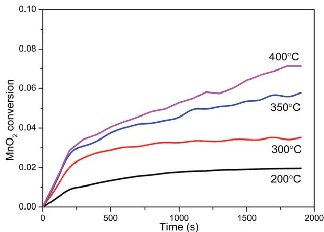
Fig. 8 Effect of temperature on solid conversion of MnO<sub>2</sub> filter at 40 Pa of SO<sub>2</sub> gas pressure.
