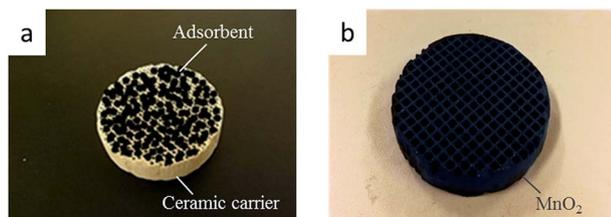
Fig. 1 Photograph of traditional filter (a) and MnO<sub>2</sub> filter (b).
