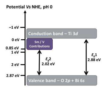
Scheme 1 Band structure of SBVT, relative to NHE at pH  $_{
