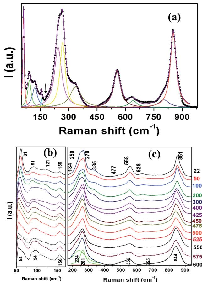
Fig. 4 (a) Normalized Raman spectra of SBVT measured at room temperature. Temperature evolution of Raman spectra obtained in the frequency range 50–170  $\text{cm}^{-1}$  (b) and 170–940  $\text{cm}^{-1}$  (c).
