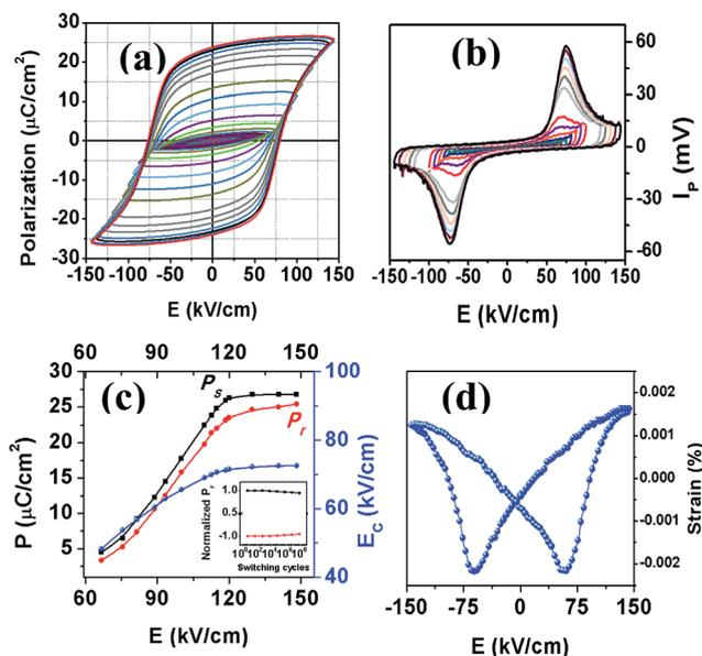
Fig. 8 Room temperature polarization–electric field hysteresis loops of SBVT. Inset: electric field dependence of polarization current. (b)  $P_r$  vs. electric field. (c) Room temperature piezoelectric strain loop of SBVT at 1 Hz. Inset (c): normalized  $P_r$  as a function of switching cycles. Comparison of  $P$ - $E$  loops before and after  $10^8$  cycles is presented in fig. S4.† (d) Piezoelectric strain vs. electric field.
