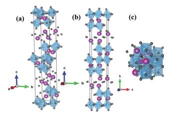
Fig. 2 (a) 3D rendering of SBVT, in the ball-and-stick and polyhedron models, obtained using the structural data extracted from GSAS. (b) Along the a-axis direction; (c) along the c-axis direction. In the 3D renderings, the small dark grey spheres represent oxygen, the bigger light-blue sphere titanium, whilst the bigger violet spheres bismuth (in it is shown the fraction of samarium, magenta color).
