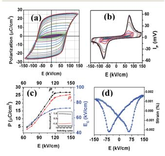
Fig. 8 Room temperature polarization-electric field hysteresis loops of SBVT. Inset: electric field dependence of polarization current. (b) Pr vs. electric field. (c) Room temperature piezoelectric strain loop of SBVT at 1 Hz. Inset of (c): normalized  $P_r$  as a function of switching cycles. Comparison of P-E loops before and after  $10^8$  cycles is presented in fig. S4.† (d) Piezoelectric strain vs. electric field.
