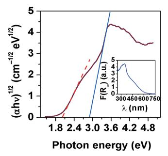
Fig. 11 Kubelka–Munk elaboration *versus* photon energy according to the indirect  $E_{\rm g}$  model ( $\gamma=2$ ). The blue line and the dashed red line represent the x-axis intercept of the line that is tangent to the inflection points of the curve (i.e. apparent optical indirect  $E_{\rm g}$ s as calculated using the Tauc procedure). In the inset is reported the DRS spectrum of SBVT.
