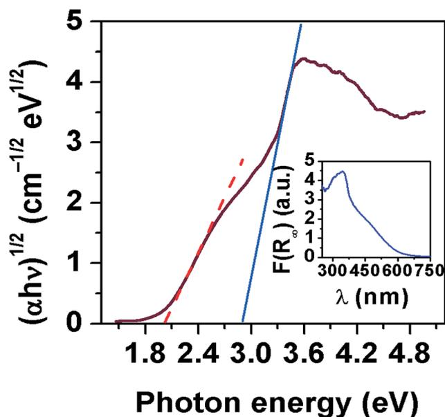
Fig. 11 Kubelka–Munk elaboration versus photon energy according to the indirect  $E_g$  model ( $\gamma = 2$ ). The blue line and the dashed red line represent the x-axis intercept of the line that is tangent to the inflection points of the curve (i.e. apparent optical indirect  $E_g$ s as calculated using the Tauc procedure). In the inset is reported the DRS spectrum of SBVT.
