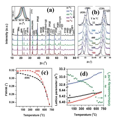
Fig. 3 (a) HTXRD  $\theta$ -2 $\theta$  scans of SBVT sample measured in the 2 $\theta$  range of 10–80°. Temperature dependent changes in the profiles of (020)/(200) and (220)/(1115) reflections (b), FWHM of (020)/(200) peaks (c) and unit cell parameters (d). Arrow in (d) indicates the phase transition temperature
