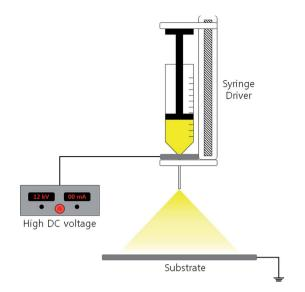
**Fig. 2** Schematic illustration of the preparation for the electrospun PVDF-*co*-HFP membrane.
