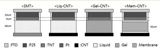
Fig. 3 Schematic illustration of DSSCs fabricated with Pt and MWCNT-based CE in combination of various types of electrolytes.
