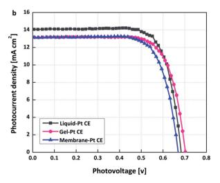
Fig. 12 Polarization curve of DSSCs fabricated with different electrolyte types in a combination of (a) MWCNT- and (b) Pt-based CEs under 1 sun illumination.
