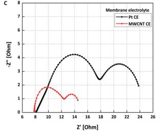
Fig. 11 Nyquist plot obtained for symmetrical cells of Pt- and MWCNT-based CEs fabricated with (a) a liquid, (b) a gel polymer and (c) a fibrous membrane electrolyte.
