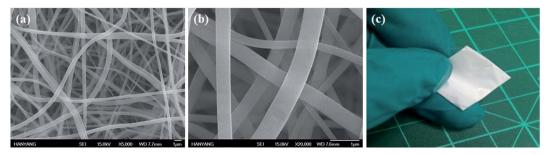
Fig. 5 FE-SEM image of the electrospun PVdF-co-HFP membrane used as the pore-filled electrolyte
