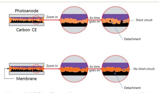
Fig. 1 Schematic illustration of a MWCNT-based CE and pore-filled membrane electrolyte demonstrating the possibility of no short circuits in cells.
