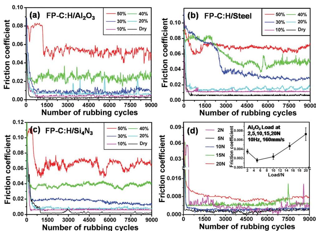
Fig. 3 (a–c) The friction coefficient curves as a function of rubbing cycles at different humidity against  $\text{Al}_2\text{O}_3$ ,  $\text{Si}_4\text{N}_3$ , and steel ball, respectively. (d) Friction coefficient curves of the FP-C:H films in a dry air atmosphere under a load from 2 N to 20 N, the inset shows the friction coefficient as a function of load.
