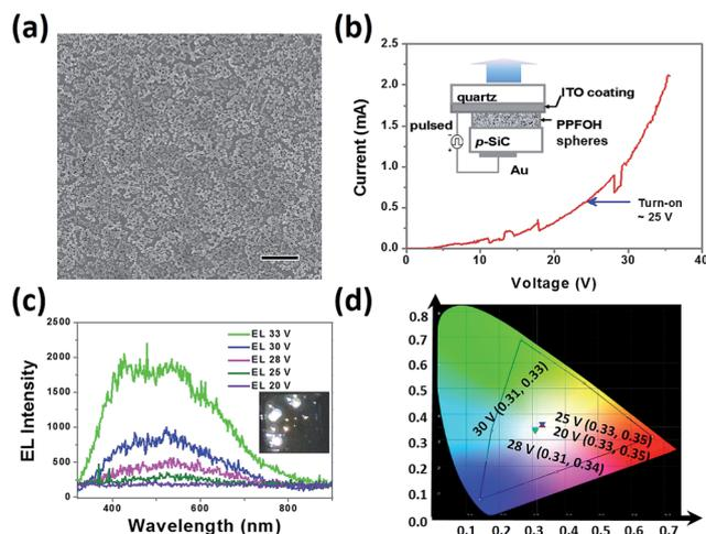
Fig. 3 (a) SEM images of the PPF OH-based films on the p-SiC, scale bar is 5  $\mu\text{m}$ . (b) Current–voltage ( $I$ – $V$ ) curve of the PNLEDs; the inset is the device configuration of the PNLEDs based on PPF OH spheres. (c) EL spectra at different voltages; the inset is the photograph of device with white light emission. (d) CIE coordinates of PNLEDs biased at various voltages.
