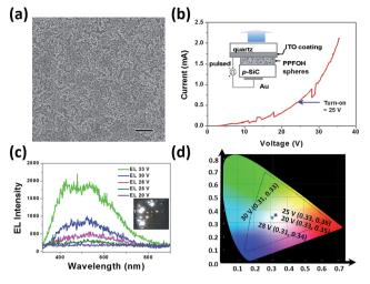
Fig. 3 (a) SEM images of the PPFOH-based films on the p-SiC, scale bar is 5  $\mu$ m. (b) Current-voltage (I-V) curve of the PNLEDs; the inset is the device configuration of the PNLEDs based on PPFOH spheres. (c) EL spectra at different voltages; the inset is the photograph of device with white light emission. (d) CIE coordinates of PNLEDs biased at various voltages
