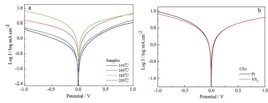
Fig. 3 Tafel curves for (a) various VS<sub>2</sub> CEs and (b) the Pt CE and the VS<sub>2</sub> CE prepared at 180 °C.
