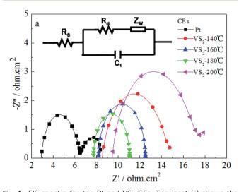
Fig. 4 EIS spectra for the Pt and  ${\rm VS_2}$  CEs. The inset (a) shows the equivalent circuit model used for fitting the resultant impedance spectra.
