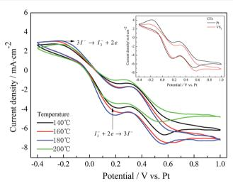
Fig. 2 Cyclic voltammograms for the Pt and VS<sub>2</sub> (prepared at 140 °C to 200 °C) CEs.
