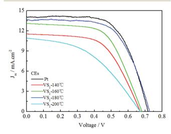
Fig. 5 Photocurrent density–voltage curves of the DSSCs based on Pt and various  $VS_2$  CEs.
