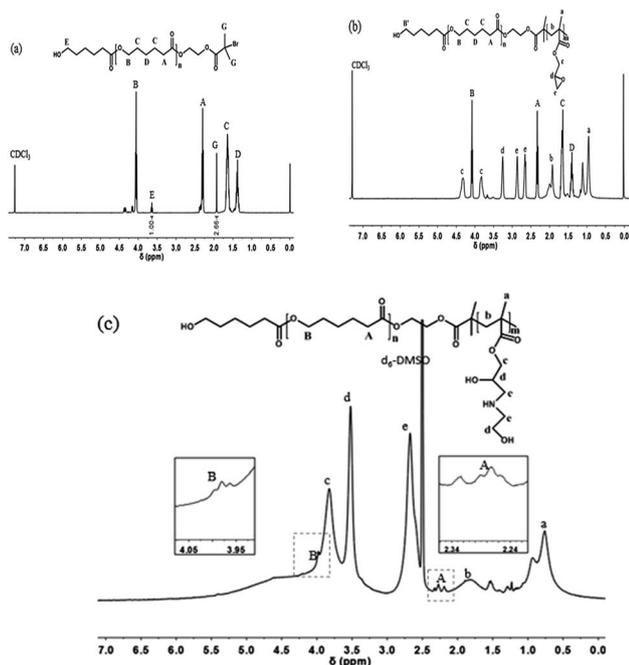
Fig. 1 The  $^1\text{H}$  NMR (400 MHz) spectra of (a) PCL-Br (b) PCL-*b*-PGMA<sub>60</sub> and (c) PCL-*b*-PGMA<sub>142</sub>.
