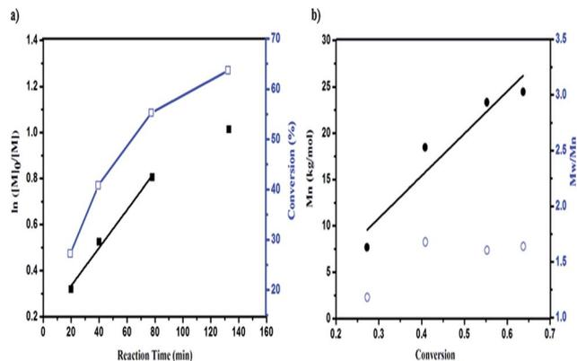
Fig. 3 The DhHP-6 catalyzed AGET ATRP of GMA using the macro-initiator PCL-Br. (a) First-order kinetic plots for semilogarithmic kinetic plot of  $\ln([M]_0/[M])$  (■) and conversion (□) as a function of reaction time. (b)  $M_n$  (●) and  $M_w/M_n$  (○) as a function of the monomer conversion. Note:  $[M] : [I] : [C] : [Asc] = 124 : 1 : 1 : 0.5$ .
