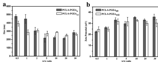
Fig. 5 The particle size and surface zeta potential of PCL-*b*-PGEA<sub>60</sub> and PCL-*b*-PGEA<sub>142</sub> in serum free condition at various w/w ratios. Data are shown as the mean  $\pm$  SD ( $n = 3$ ).
