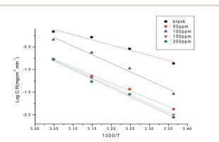
Fig. 5 Arrhenius plots (log C.R. vs. 1/T) for carbon steel in 1.0 M HCl without and with different concentrations of GRE.
