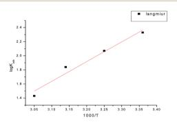
Fig. 4 Log  $K_{ads}$  vs. (1/T) curves for the corrosion of carbon steel in 1 M HCl in the absence and presence of different concentrations of GRE.
