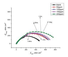
Fig. 10 Nyquist plots for the corrosion of carbon steel in 1.0 M HCl in the absence and presence of different concentrations of GRE at 25  $^{\circ}$ C.
