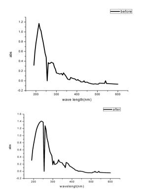
Fig. 18 UV-visible spectra of the solution from 1.0 M HCl containing 200 ppm GRE before and after 24 h of carbon steel immersion.
