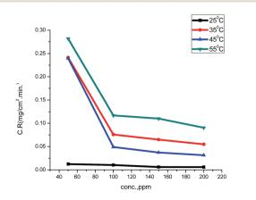
Fig. 1 Corrosion rates of various concentrations of ginger roots extract on carbon steel in 1.0 M HCl at 25–55  $^{\circ}\text{C}$
