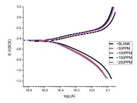
Fig. 8 Anodic and cathodic polarization curves for carbon steel in 1.0 M HCl in the absence and presence of different concentrations of GRE at 25  $^{\circ}$ C.
