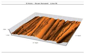
Fig. 13 Surface of polished carbon steel electrode as viewed by atomic force microscopy
