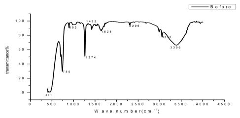
Fig. 16 FT-IR spectrum of GRE before adsorption on a carbon steel surface.
