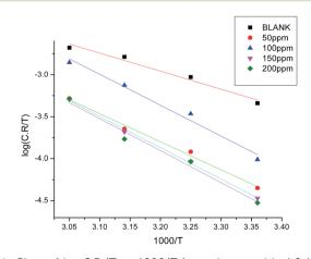
Fig. 6 Plots of log C.R./T vs. 1000/T for carbon steel in 1.0 M HCl without and with different concentrations of GRE.
