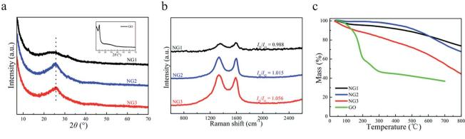
Fig. 2 XRD patterns (a), Raman spectra (b) and TGA curves (c) of NG1, NG2 and NG3.
