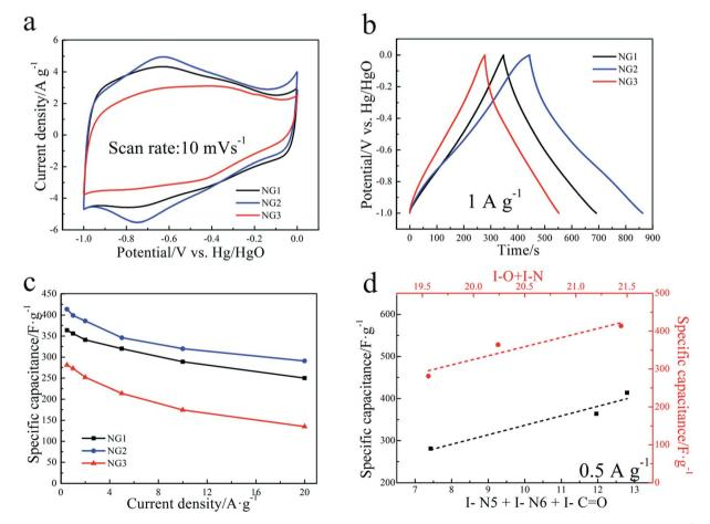
Fig. 4 Electrochemical performance of the samples in three-electrode system. (a) The CV curves of NGs at a scanning rate of 10 mV s<sup>-1</sup>; (b) the GCD curves of NGs at a current densities of  $1 \text{ A g}^{-1}$ ; (c) the specific capacitance at various current densities of NGs; (d) specific capacitance as a function of the sum of nitrogen and oxygen content (red line) and the sum of I-N5, I-N6, I-C=O content (black line) at 0.5 A  $g^{-1}$ .
