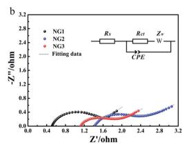
Fig. 5 (a) Nyquist plot of NGs, (b) AC impedance plots and the equivalent circuit for NGs electrodes.
