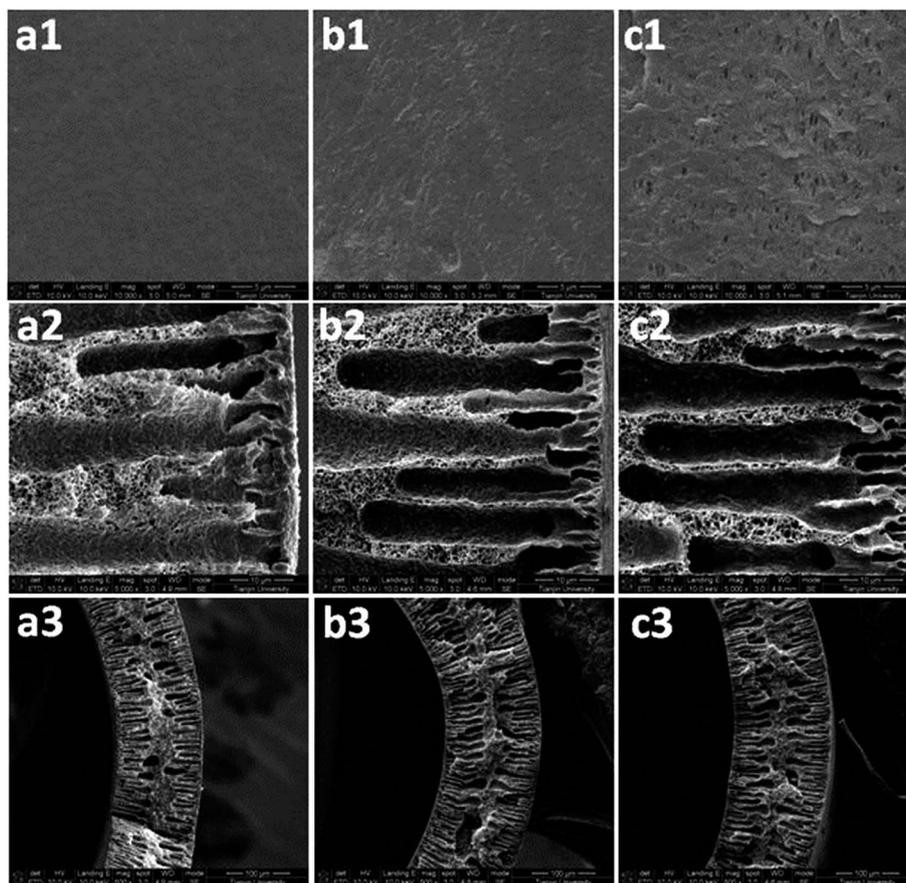
Fig. 6 FE-SEM images of the outer surface and cross-section of the PVDF membranes: (a) new membrane, (b) control membrane, and (c) test membrane.
