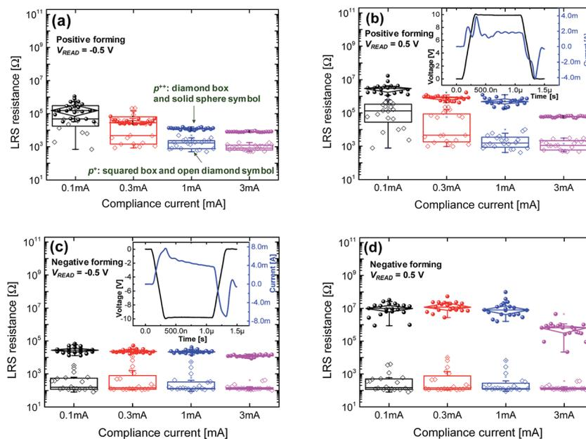
Fig. 3 (a) Statistical distribution of the LRS resistance for the Ni/SiN<sub>x</sub>/p<sup>++</sup> Si device and Ni/SiN<sub>x</sub>/p<sup>+</sup> Si device: read voltage of  $-0.5$  V (a), and  $0.5$  V (b) for positive forming; and read voltage of  $-0.5$  V (c), and  $0.5$  V (d) for negative forming. The insets of (b) and (c) show the transient characteristics of positive forming and negative forming, respectively, for the Ni/SiN<sub>x</sub>/p<sup>+</sup> Si device.
