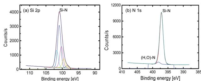
Fig. 1 XPS spectra of the SiN<sub>x</sub> film deposited *via* LPCVD: (a) Si 2p and (b) N 1s.
