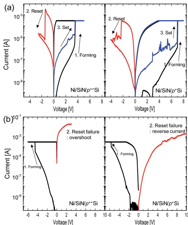
Fig. 2 (a) Typical *I*–*V* curves of the Ni/SiN<sub>x</sub>/p<sup>++</sup> Si device (left) and Ni/SiN<sub>x</sub>/p<sup>+</sup> Si device (right); electroforming at (a) positive voltage, and (b) negative voltage.
