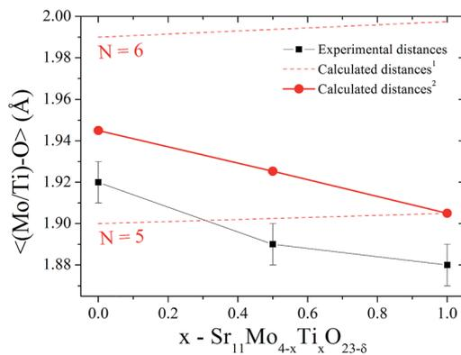
Fig. 4 Experimental and theoretical distances for the (Mo/Ti)–O bond taking into account the Mo/Ti ratio, and the coordination number. <sup>1</sup>Calculated distances taking into account a coordination number of  $N = 6$  or  $5$ . <sup>2</sup>Calculated distances taking into account an effective coordination number of  $N = 5.5, 5.25$  and  $5$  expected for  $x = 0, 0.5$  and  $1.0$ , respectively.
