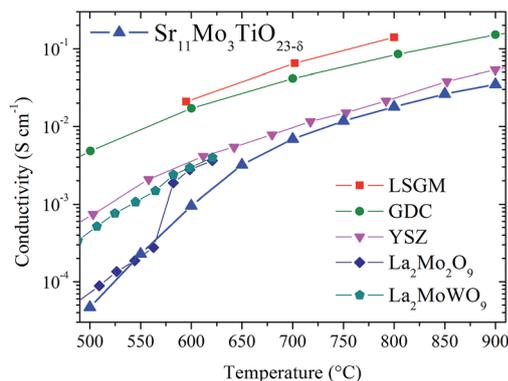
Fig. 12 Values of conductivity of  $\text{Sr}_{11}\text{Mo}_3\text{TiO}_{23-\delta}$  in comparison with LSGM, GDC, YSZ,  $\text{La}_2\text{Mo}_2\text{O}_9$  and  $\text{La}_2\text{MoWO}_9$ .<sup>27–31</sup>
