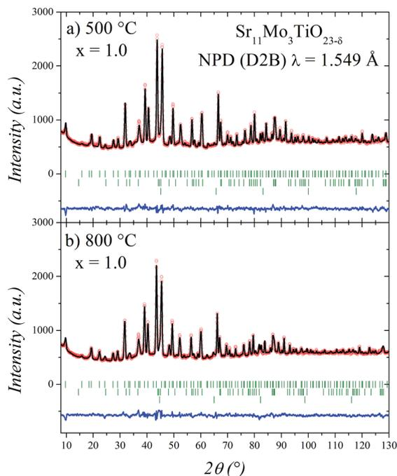
Fig. 5 Observed (circles), calculated (full line) and difference (bottom) Rietveld profiles at (a) 500 °C and (b) 800 °C for  $\text{Sr}_{11}\text{Mo}_3\text{TiO}_{22}$  after NPD refinement. The second and third series of tick marks correspond to the Bragg reflections for  $\text{SrMoO}_4$  and  $\text{Sr}_2\text{TiO}_4$  impurities, respectively.
