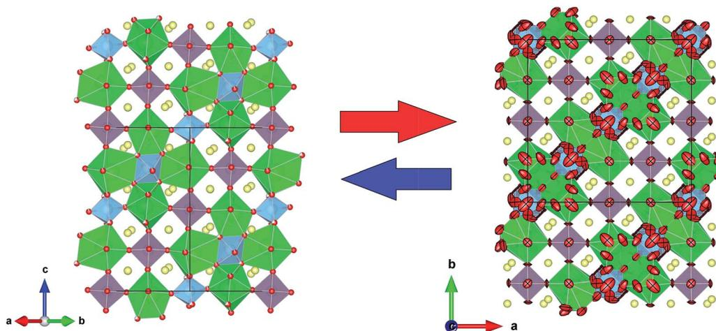
Fig. 8 Schematic view of crystal structure at room temperature (left) and at 800 °C (right) for  $x = 1$ . Both structures are shown in equivalent projections: along [110] and [001] for tetragonal (left) and cubic (right) symmetries, respectively.
