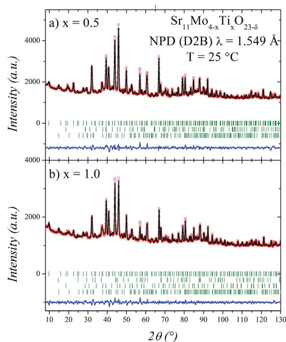
Fig. 2 Observed (circles), calculated (full line) and difference (bottom) Rietveld profiles at room temperature for  $\text{Sr}_{11}\text{Mo}_{4-x}\text{Ti}_x\text{O}_{23-\delta}$  with  $x = 0.5$  (a) and  $1.0$  (b) after NPD refinement at RT. The lower series of tick marks correspond to the Bragg reflections for impurities in the same order that is shown in XRPD refinements.
