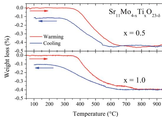
Fig. 10 TGA curves of doped samples  $\text{Sr}_{11}\text{Mo}_{4-x}\text{Ti}_x\text{O}_{23-\delta}$  with  $x = 0.5$  (top panel) and 1.0 (bottom panel). Red lines correspond to warming and blue lines to cooling.
