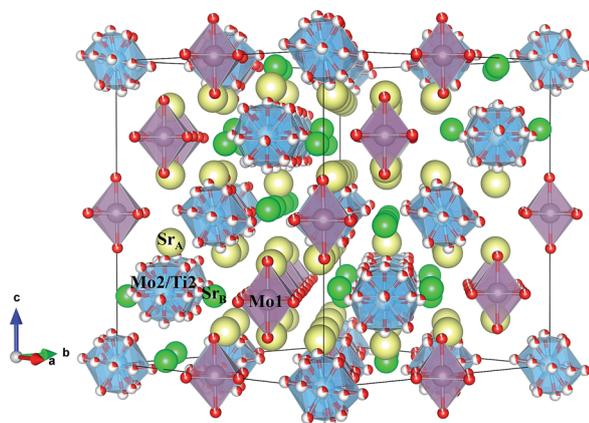
Fig. 6 Schematic view of the cubic crystal structure (800 °C) showing Mo1 octahedra and Mo2/Ti2 polyhedra.
