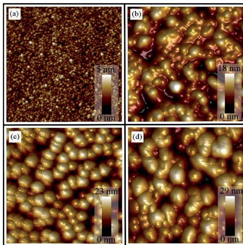
Fig. 9 (Top two) AFM images ( $1 \times 1 \mu\text{m}^2$ ) of a compressively ( $0.8$  GPa) stressed (111) YSZ films on Si (a) as-deposited, (b) annealed respectively. (Bottom two) AFM images ( $1 \times 1 \mu\text{m}^2$ ) of a tensile stressed ( $0.2$  GPa) stressed (100) YSZ films on Si (c) as-deposited, (d) annealed respectively. Line profile on the AFM images provided information on grain sizes.
