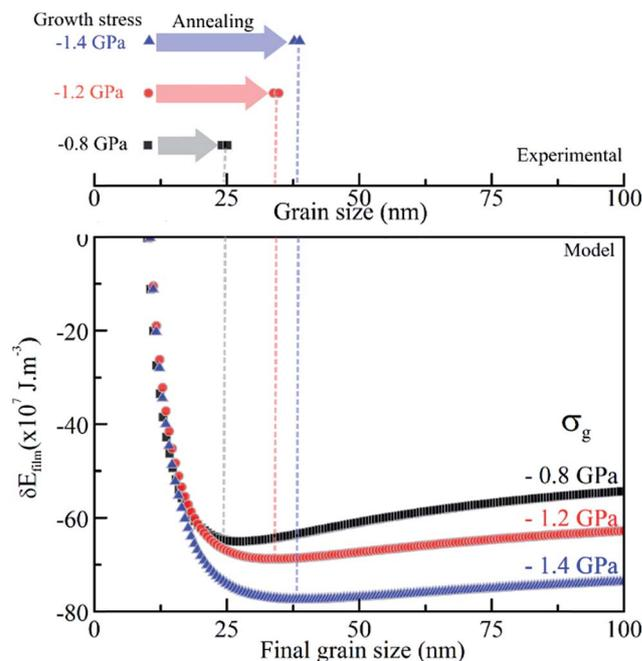
Fig. 11 Change in film energy *versus* final grain size plots, for three (111) YSZ films with  $d_0 < d_{\text{cr}}$ , show energy minima as expected from model. The corresponding top figure shows the final grain sizes after twice annealing and also indicates that grain growth get saturated at their energy minima.
