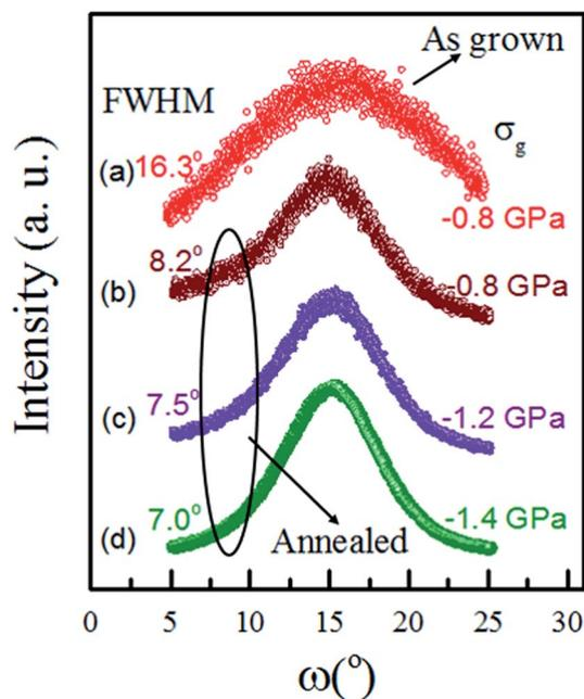
Fig. 6 XRD ( $\omega$ ) scans of (111) YSZ films of one as-grown with  $-0.8$  GPa growth stress and some annealed ones with  $-0.8$ ,  $-1.2$  and  $-1.4$  GPa growth stresses. These plots show reduction in FWHM of rocking curves for higher compressive stressed films after annealing.
