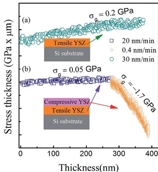
Fig. 4 Stress thickness *vs.* thickness plots show *in situ* stresses in (100) YSZ films (a) a tensile stressed (grown at  $30 \text{ nm min}^{-1}$ ) and (b) a stack of two layers—a compressive layer (at  $0.4 \text{ nm min}^{-1}$ ) on top of a tensile layer (at  $20 \text{ nm min}^{-1}$ ). Each large division is equivalent to  $0.1 \text{ GPa } \mu\text{m}$ .
