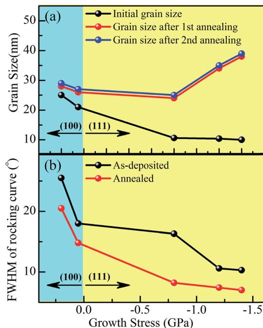
Fig. 8 (a) Grain size versus growth stress of as-deposited and annealed films plots show grain-growth on annealing (b) FWHM of rocking curve versus growth stress of as-deposited and annealed films plots show improvement in texture on annealing.
