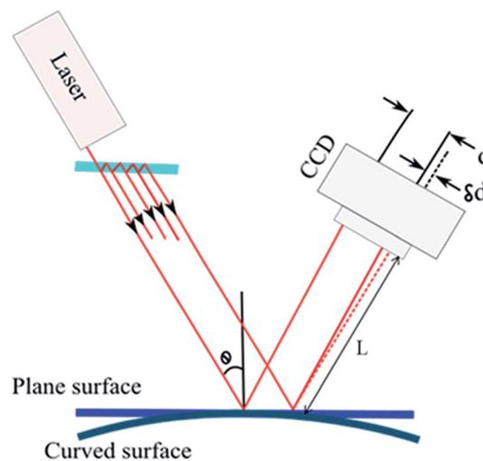
Fig. 1 Schematic of *in situ* curvature measurement during thin film growth by a multiple beam optical stress sensor (MOSS) and determination of stress from the change in curvature by Stoney's equation.
