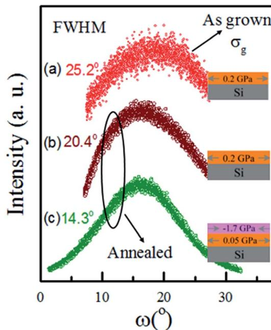
Fig. 7 XRD ( $\omega$ ) scans of (100) YSZ films for a tensile stressed (a) as-deposited and (b) annealed film with  $0.2$  GPa stress, (c) for an annealed film composed of two layers, a compressive layer ( $-1.7$  GPa) on a tensile layer ( $0.05$  GPa).
