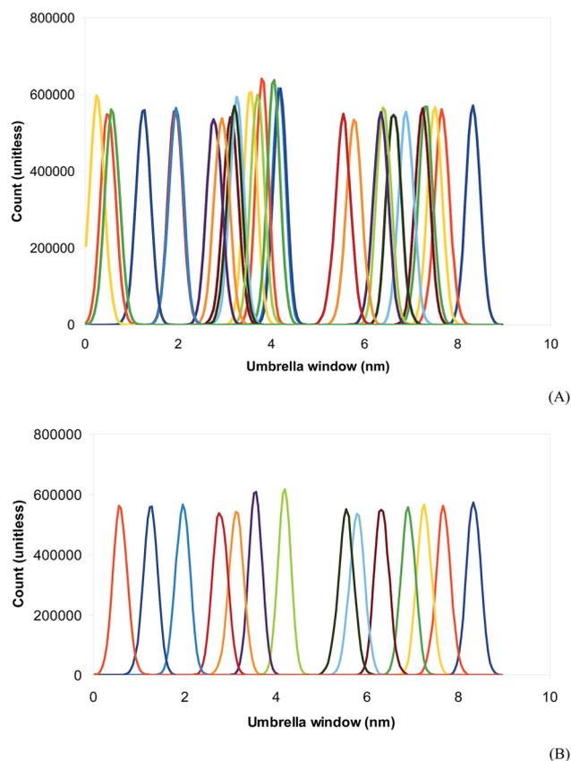
**Fig. 6** The weighted histogram analysis of the overlap between umbrella windows from 0 to 9 nm in the reaction coordinate. (A) All umbrella windows. (B) Only selected umbrella windows. There is no meaning in each color. The only importance is a better visualization of the overlapping.
