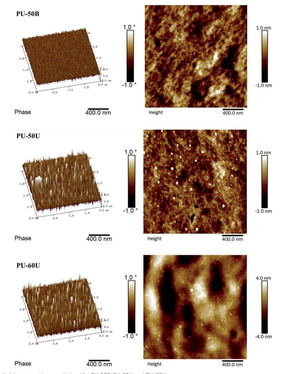
Fig. 5 Phase/height contrast images obtained for PU-50B, PU-50U, and PU-60U.
