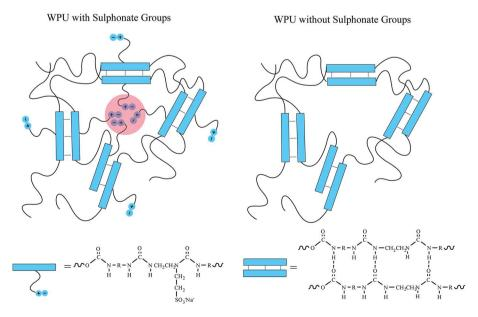
Scheme 1 Comparison of the dual self-healing polyurethane system with sulphonate groups and hydrogen bonds and without sulphonate groups.
