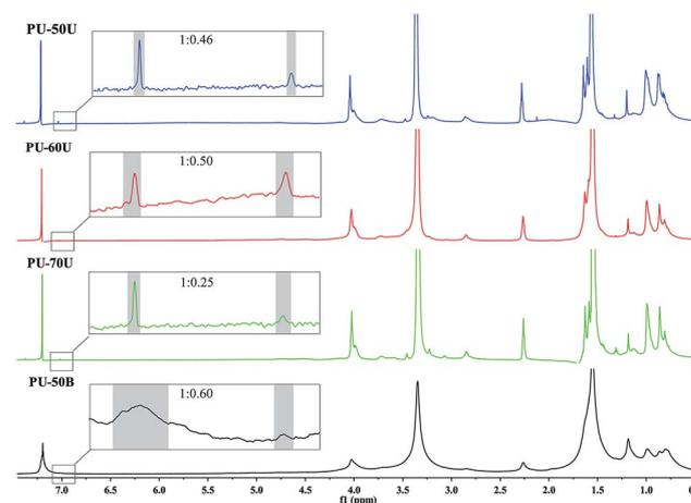
Fig. 2  $^1\text{H-NMR}$  spectra of the pure WPUs.
