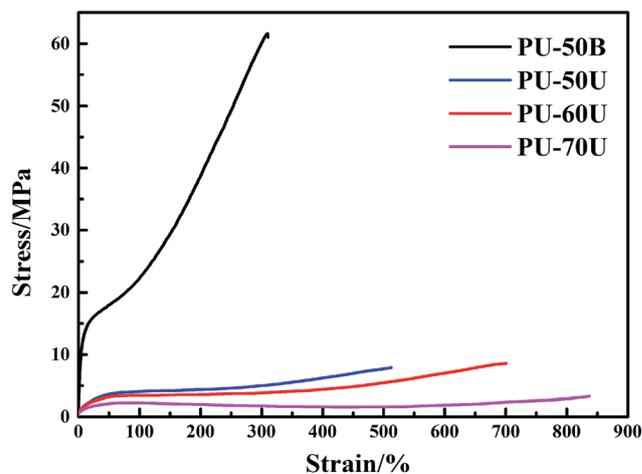
Fig. 7 Stress–strain curves of the different WPU films.
