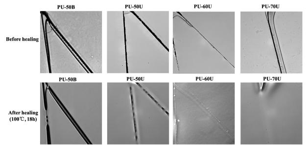
Fig. 4 Optical microscope images of PU-50B, PU-50U, PU-60U, and PU-70U before healing and after healing (100 °C, 18 h).
