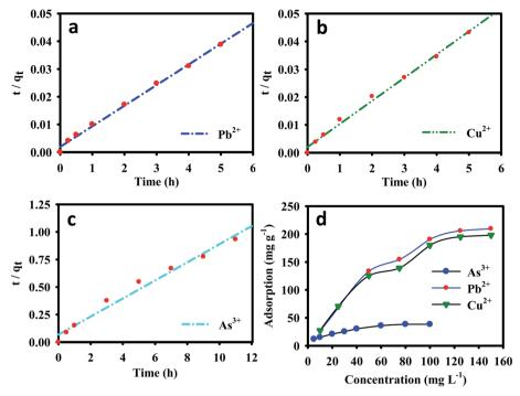
Fig. 3 Pseudo-second-order curve-fitting graphs of (a)  $Pb^{2+}$ , (b)  $Cu^{2+}$ , and (c)  $As^{3+}$  at 298.15 K. (d) Adsorption profiles of  $Pb^{2+}$ ,  $Cu^{2+}$ , and  $As^{3+}$  on EDTA-MCS/GO nanocomposite at different metal ion concentrations.
