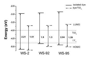
Fig. 5 The molecular energy level diagrams of the dyes and dye/ ${\rm TiO_2}$  systems in the gas phase.
