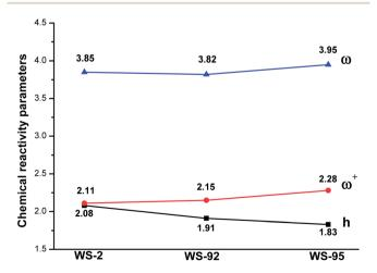
Fig. 11 Chemical hardness, electrophilicity index, and electron accepting power of the dyes
