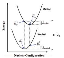
Fig. 2 Calculation of the hole reorganization energy.
