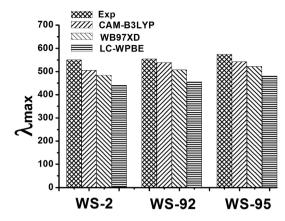
Fig. 8 The effects of different functionals on the absorption maxima  $(\lambda_{max}/nm)$  of the dyes in CH<sub>2</sub>Cl<sub>2</sub> solution.
