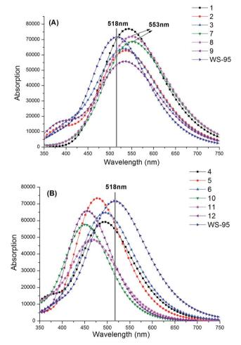
Fig. 13 Absorption spectra of the designed molecules and the reference dye WS-95 ((A) represents dyes with the insertion of -CN, (B) represents dyes with the insertion of  $-NH_2$ ).
