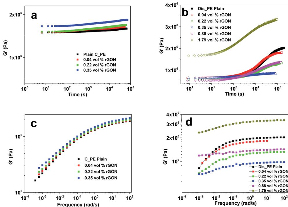
Fig. 7 Storage modulus vs. frequency graphs of (a) C\_PE/rGON composites. (b) Dis\_PE/rGON composites and frequency sweep graphs of (c) C\_PE/rGON composites. (d) Dis\_PE composites (reproduced with permission from ref. 79 copyright 2015 American Chemical Society).
