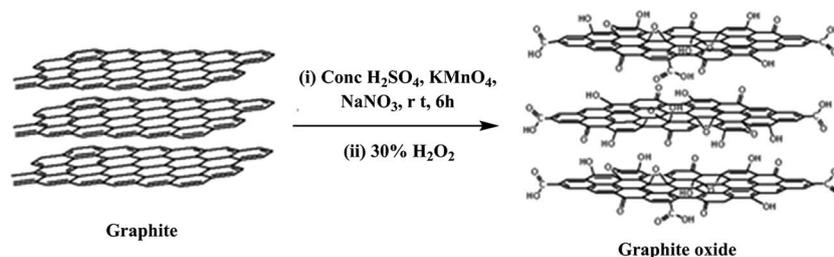
Fig. 2 Schematic representation of the oxidation of graphite to graphite oxide.
