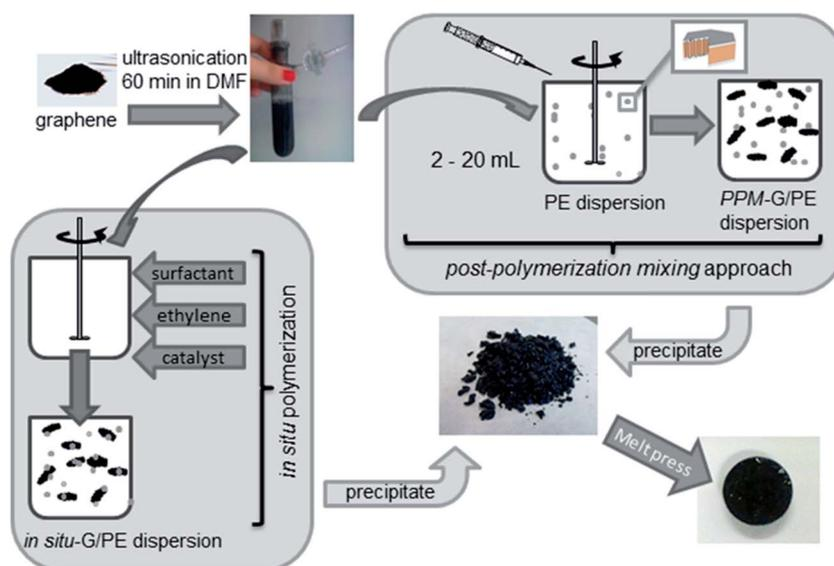
Fig. 4 Preparation of PE/graphene composites by *in situ* polymerization, post polymerization mixing and precipitation methods (reproduced with permission from ref. 58 copyright 2014 American Chemical Society).
