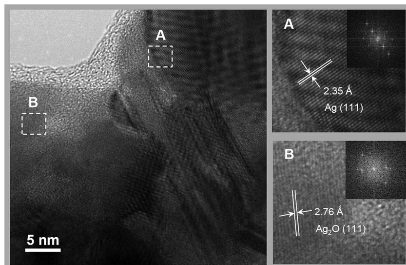
Fig. 4 HRTEM images of as-synthesized Ag NWs. The insets show the Fourier transform patterns of lattice images.
