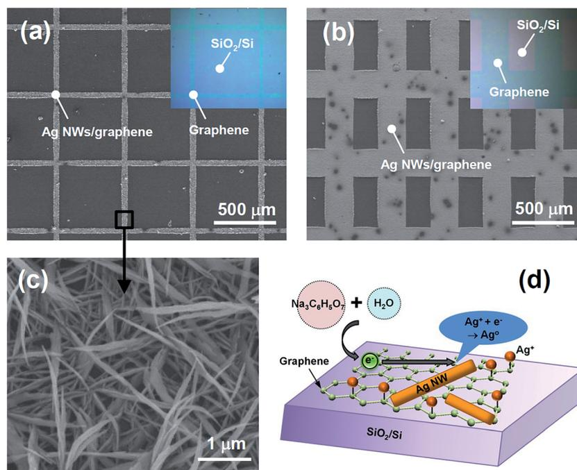
Fig. 1 SEM images of Ag NWs synthesized on pre-patterned graphene: (a) pattern A, (b) pattern B, and (c) enlarged Ag NW image. The insets show the microscope images of graphene patterns on SiO<sub>2</sub>/Si substrates. (d) Schematic diagram of Ag NWs on graphene synthesized using a modified citrate reduction reaction.
