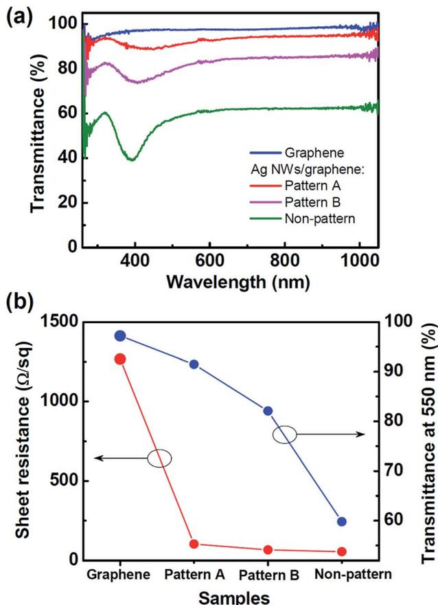
Fig. 7 (a) Light transmittance spectra and (b) sheet resistance and light transmittance at 550 nm of pristine graphene, and pattern A, pattern B, and non-patterned samples of graphene–Ag NW films.
