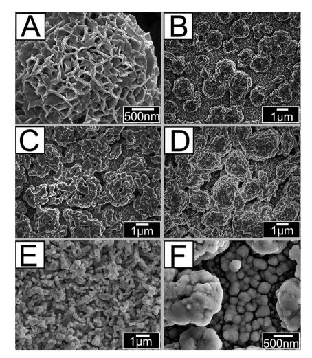
Fig. 1 SEM patterns of: (A) the Bi<sub>2</sub>MoO<sub>6</sub> before annealing, (B) BM-20, (C) BM-30, (D) BM-40, (E) CdS, and (F) Bi<sub>2</sub>MoO<sub>6</sub> & CdS composites.
