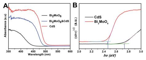
Fig. 5 (A) The UV-vis absorption spectra of the  $Bi_2MoO_6$ , CdS, and  $Bi_2MoO_6$  & CdS electrodes; (B) the band gap of CdS and  $Bi_2MoO_6$ .
