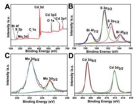
Fig. 4 The X-ray photoelectron spectroscopy (XPS) spectra of Bi<sub>2</sub>MoO<sub>6</sub> & CdS composite photoanode.
