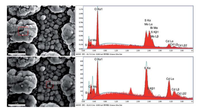
Fig. 2 The EDX patterns of Bi<sub>2</sub>MoO<sub>6</sub> & CdS composites.
