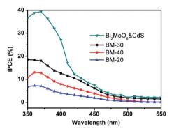
Fig. 8 The incident photon-to-current conversion efficiency (IPCE) of BM-20, BM-30, BM-40, and Bi<sub>2</sub>MoO<sub>6</sub> & CdS.
