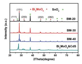
Fig. 3 XRD patterns of the BM-20, BM-30, BM-40, and  $\rm Bi_2MoO_6$  & CdS composite photoanodes samples.
