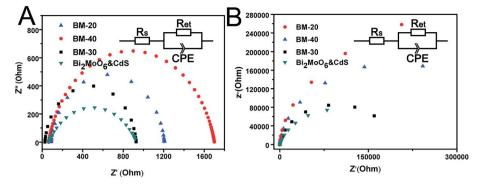
Fig. 7 Electrochemical impedance spectroscopy (EIS) Nyquist plots of BM-20, BM-30, BM-40, and Bi<sub>2</sub>MoO<sub>6</sub> & CdS composite photoanodes samples
