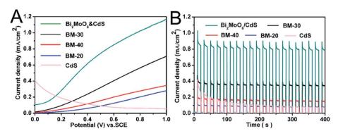
Fig. 6 (A) Linear sweep voltammograms of BM-20, BM-30, BM-40, and  $Bi_2MO_6$  & CdS composite photoanode samples in visible light illumination (100 mW cm<sup>-2</sup>); (B) amperometric I-t curves of BM-20, BM-30, BM-40, and  $Bi_2MO_6$  & CdS composite photoanodes samples.
