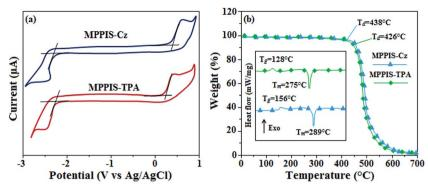
Fig. 6 (a) Cyclic voltammogram of MPPIS-Cz and MPPIS-TPA; (b) DSC and TGA graphs of MPPIS-TPA and MPPIS-Cz.
