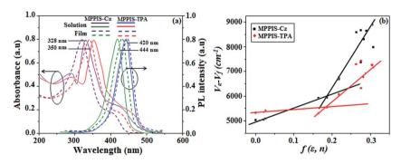
Fig. 7 (a) Normalized absorption and emission spectra of MPPIS-Cz and MPPIS-TPA in dichloromethane and film; (b) Lippert–Mataga plot of MPPIS-Cz and MPPIS-TPA in different solvents.
