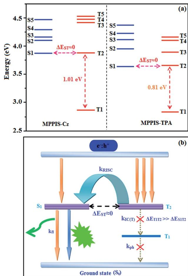
Fig. 4 (a) Energy level of singlet (S) and triplet (T) states of MPPIS-Cz and MPPIS-TPA; (b) scheme of exciton decay process after hole and electron recombination in OLEDs of twisting D- $\pi$ -A molecules.
