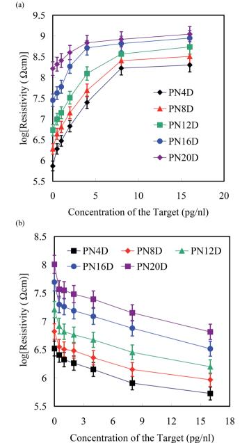
Fig. 5 Resistivities of PNIPAAm-b-ssDNA copolymer brushes (logarithm scale) plotted with respect to the hybridization concentration of the target (0.5–16 pg nL $^{-1}$ ) at (a) 25 and (b) 80 °C.
