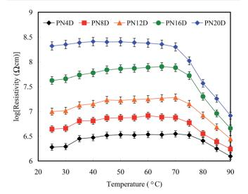
Fig. 4 Resistivities of the PNIPAAm-b-DNA copolymer brushes (logarithm scale) recorded with respect to temperature at 25 to 90  $^{\circ}$ C.
