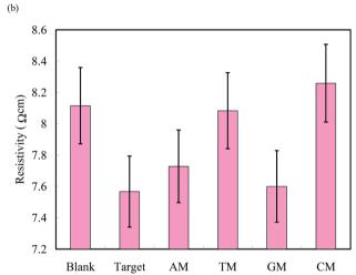
Fig. 6 Resistivities (logarithm scale) of (a) PN4D at 25  $^{\circ}$ C and (b) PN20D at 80  $^{\circ}$ C before and after hybridization with the target, AM, TM, GM, and CM at 0.5 pg nL $^{-1}$ .
